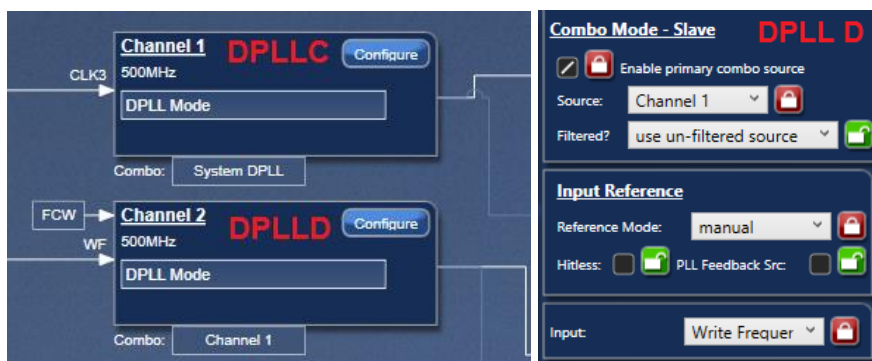
Figure 4. Receiver Side DPLLs and DPLL D FCW Configuration
