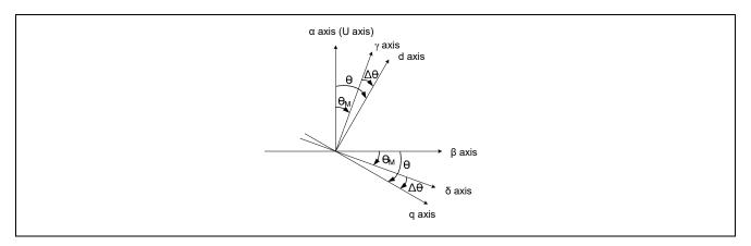
Figure 3-4 Relation between d q axis and  $\gamma \delta$  axis
