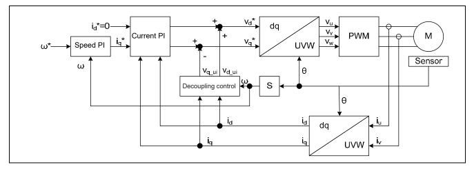
Figure 3-3 Control Flow of the Vector Control
