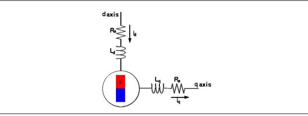
Figure 3-2 Conceptual diagram of the two phase direct current motor
