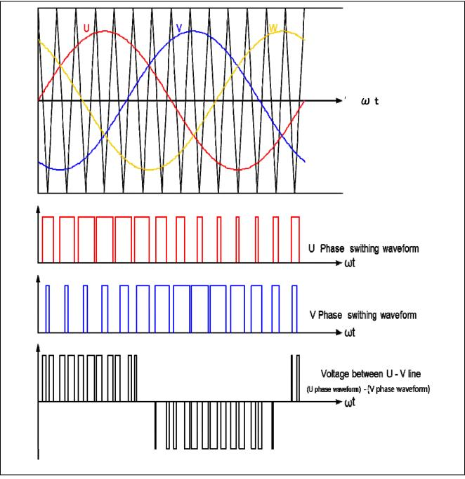
Figure 3-6 Conceptual diagram of the triangular wave comparison method
