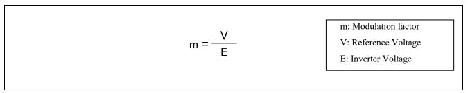
A request control can be performed by setting this modulation factor on the register which determines PWM duty.
