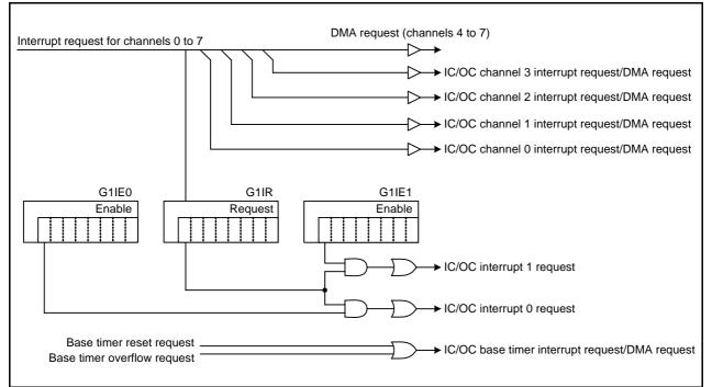
Figure 3.1 IC/OC Interrupts and DMA Request Generation
