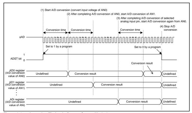
Figure 3.1 Operation Timing in Repeat Sweep Mode 0
