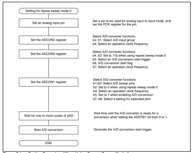
Figure 5.1 Setting Procedure When Using Repeat Sweep Mode 0
