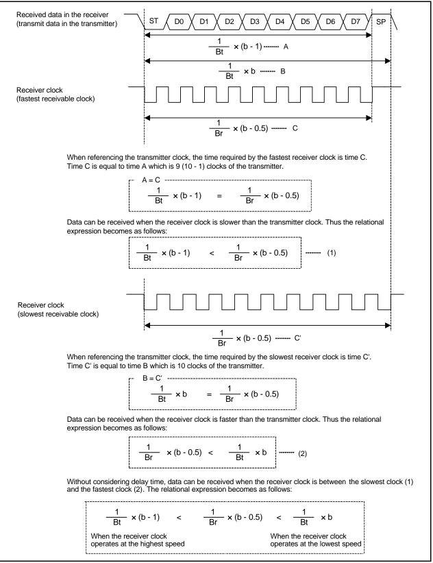
Figure 1.5 Tolerance Without Delay Time Consideration
