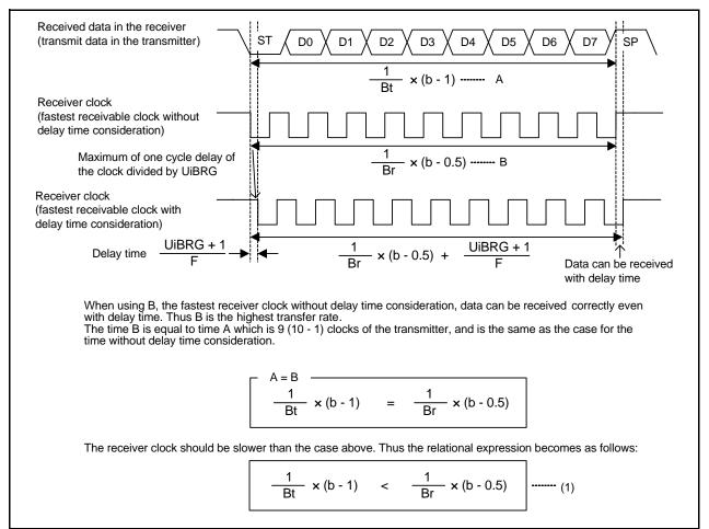
Figure 1.6 Fastest Receiver Clock with Delay Time Consideration
