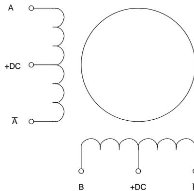
Figure 1. Unipolar Stepping Motor
