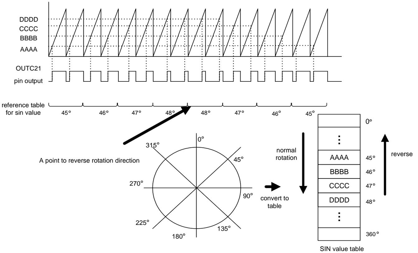
Figure 12. Control of Rotation Direction
