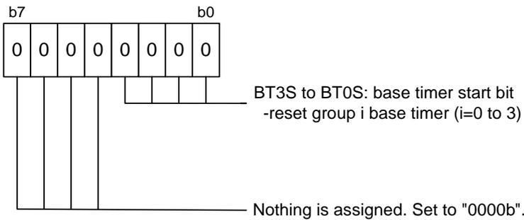
Group i base timer (i=0 to 3) is reset. After setting the base timer operation clock with the GiBCR0 register, set the BTS bit in the GiBCR1 register to "1" for the group i base timer to start counting from "0000h".
