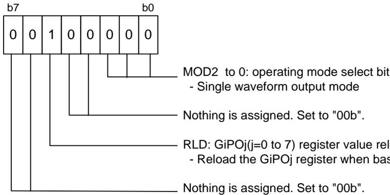
After setting the RLD bit to "1", change the reload timing of GiPO0 and GiPOj registers when the base timer is reset.
