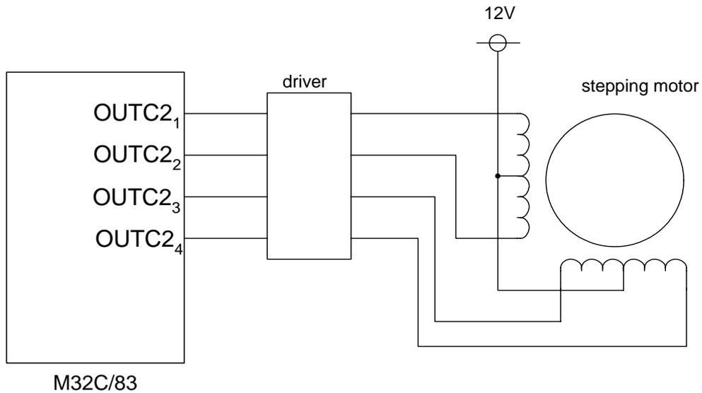
Figure 6. M32C/83 with Stepping Motor
