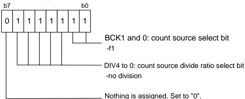
Supply to each register shown in procedures 6) to 13) and 20). To enable each register setting as soon as they are set, set the G2BCR0 register to "01111111b".
