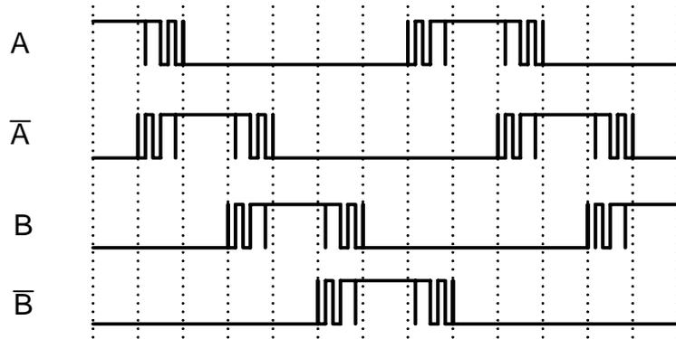
Figure 5. Microstepping Control (one-two excitation))
