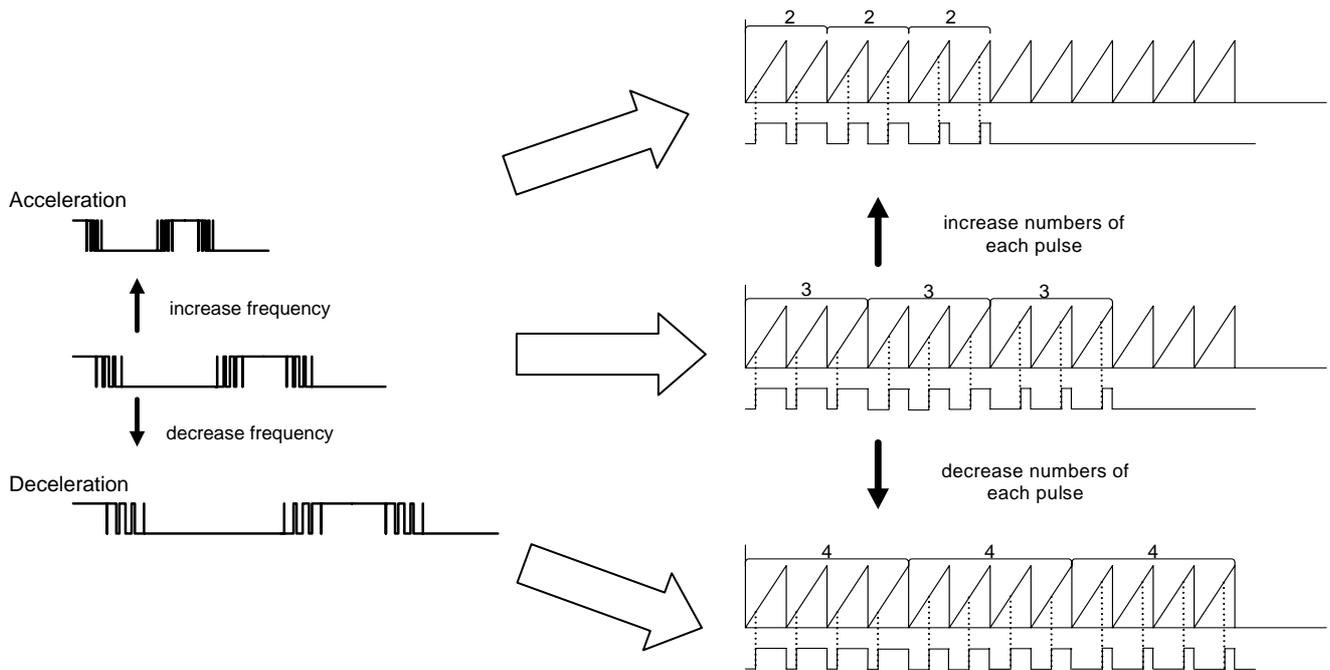
Figure 11. Changes of Stepping Motor Speed
