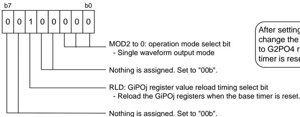
After setting the RLD bit to "1", change the reload timing of G2PO1 to G2PO4 registers when the base timer is reset.
