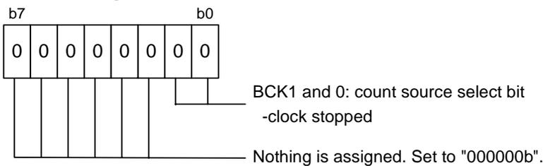
Stop supplying clocks to the group 2 base timer when the timer and the BTSR register are not used.
