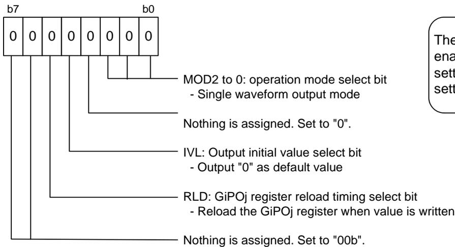
The setting of GiPO0 register is enabled as soon as it is set. When setting the GiPO0 register at initial setting, set the RLD bit to "0".
