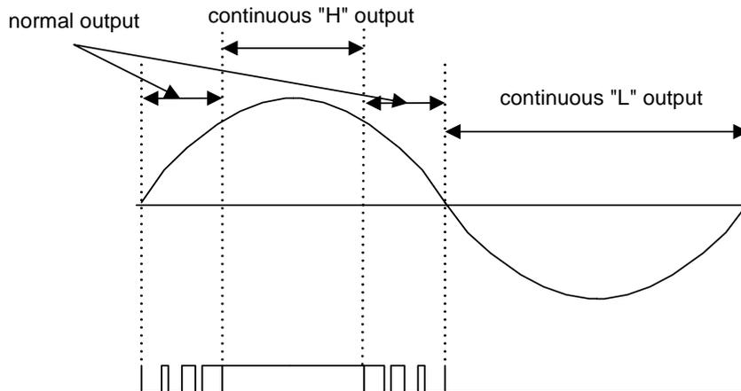
Figure 9. Sin Waveform and PWM Output
