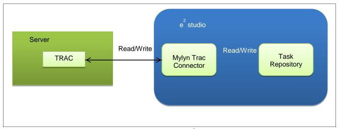
Figure 2: Architecture of Trac and e<sup>2</sup> studio co-operation
