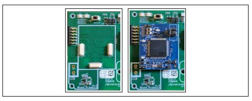
*Step 2.* Insert RL78/G1D BLE PMOD module into the PMOD connector on BPM board.
