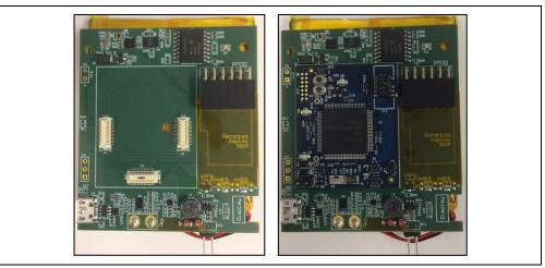
Step 2. Insert RL78/G1D BLE PMOD module into the PMOD connector on Activity board.
