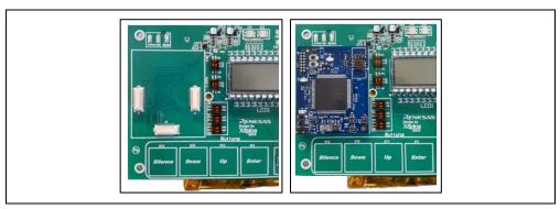
Step 2. Insert RL78/G1D BLE PMOD module into the PMOD connector on HRM/SpO2 board.
