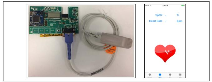
Figure 3-4 Heart Rate/Pulse Ox Module with Mobile App snapshot
