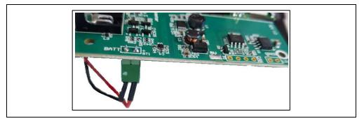
*Step 4.* Connect Pulse Oximeter Probe to board using the provided connector.
