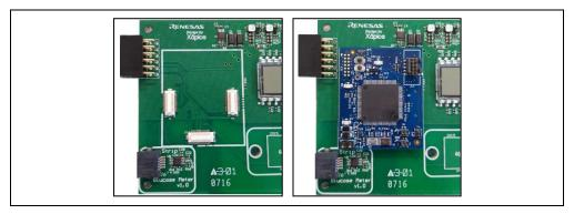
*Step 2.* Insert RL78/G1D BLE PMOD module into the PMOD connector on BGM board.
