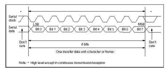
One transferred data begins with LSB and ends with the MSB. After output of the MSB, the communication line retains the MSB state. When receiving the date in synchronous mode, SCI3 latches receive data at the rising edge of the serial clock. The data transfer format uses a fixed 8-bit data length and parity and microprocessor bits cannot be added.
