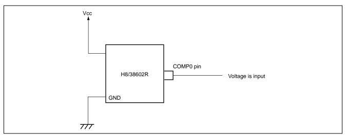
Figure 1 Connection Diagram
