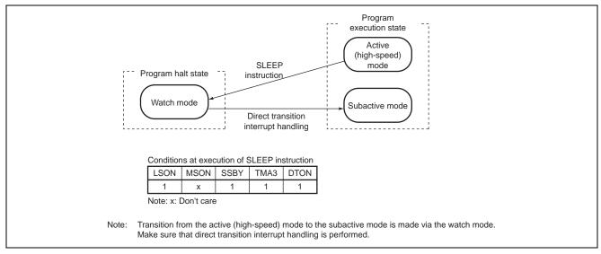
Figure 1 Mode Transition to the Subactive Mode
