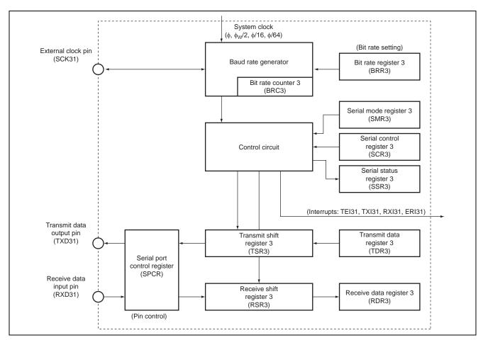
Figure 2 Block Diagram of SCI3
