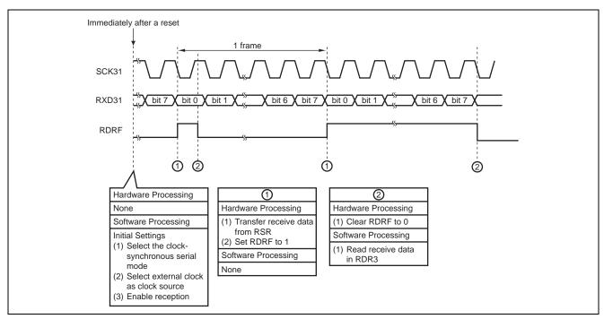
Figure 3 Principles of Operation for Serial Data Reception in the Clock-Synchronous Mode
