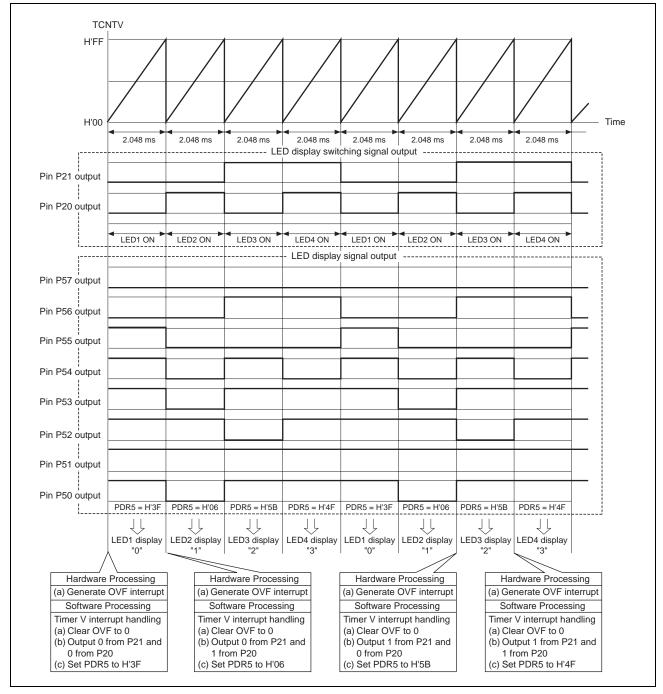
Figure 7 Operating Principle of 7-Segment LED Display Control
