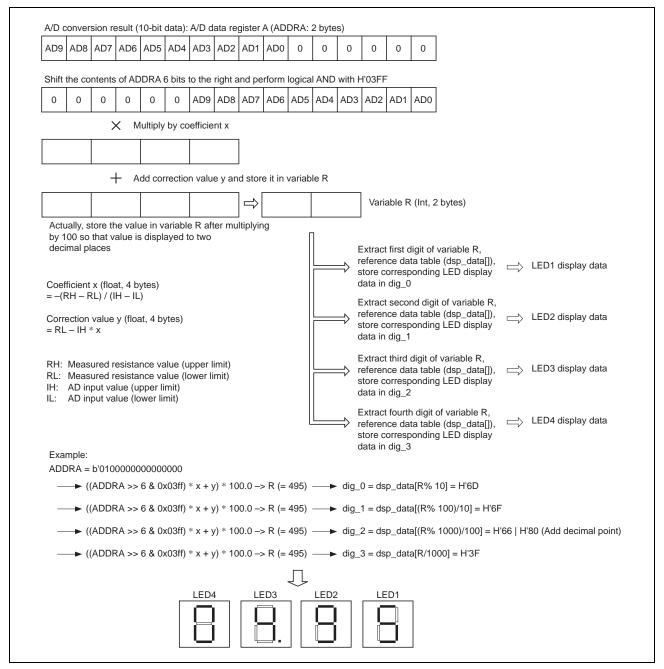
Figure 3 LED Display for A/D Conversion Result
