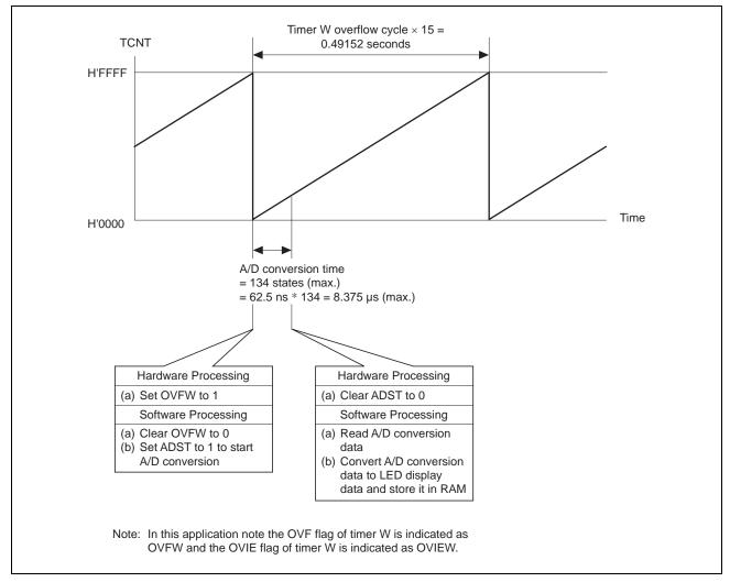
Figure 6 Operating Principle of Remote Control Reception Using Timer W
