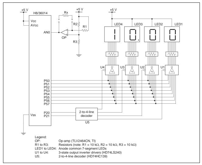
Figure 1 Hardware Configuration
