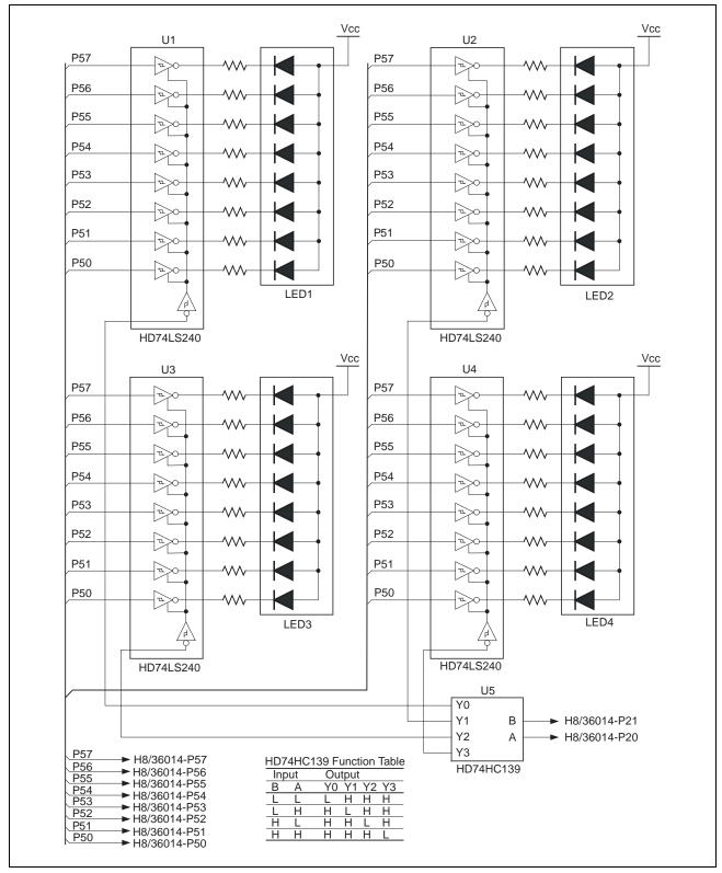
Figure 2 7-Segment LED Control Method
