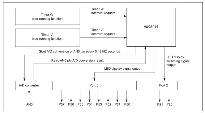
Figure 4 Block Diagram of Functions Used
