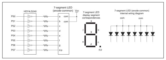
Figure 5 7-Segment LED Connection Diagram and Internal Wiring Diagram
