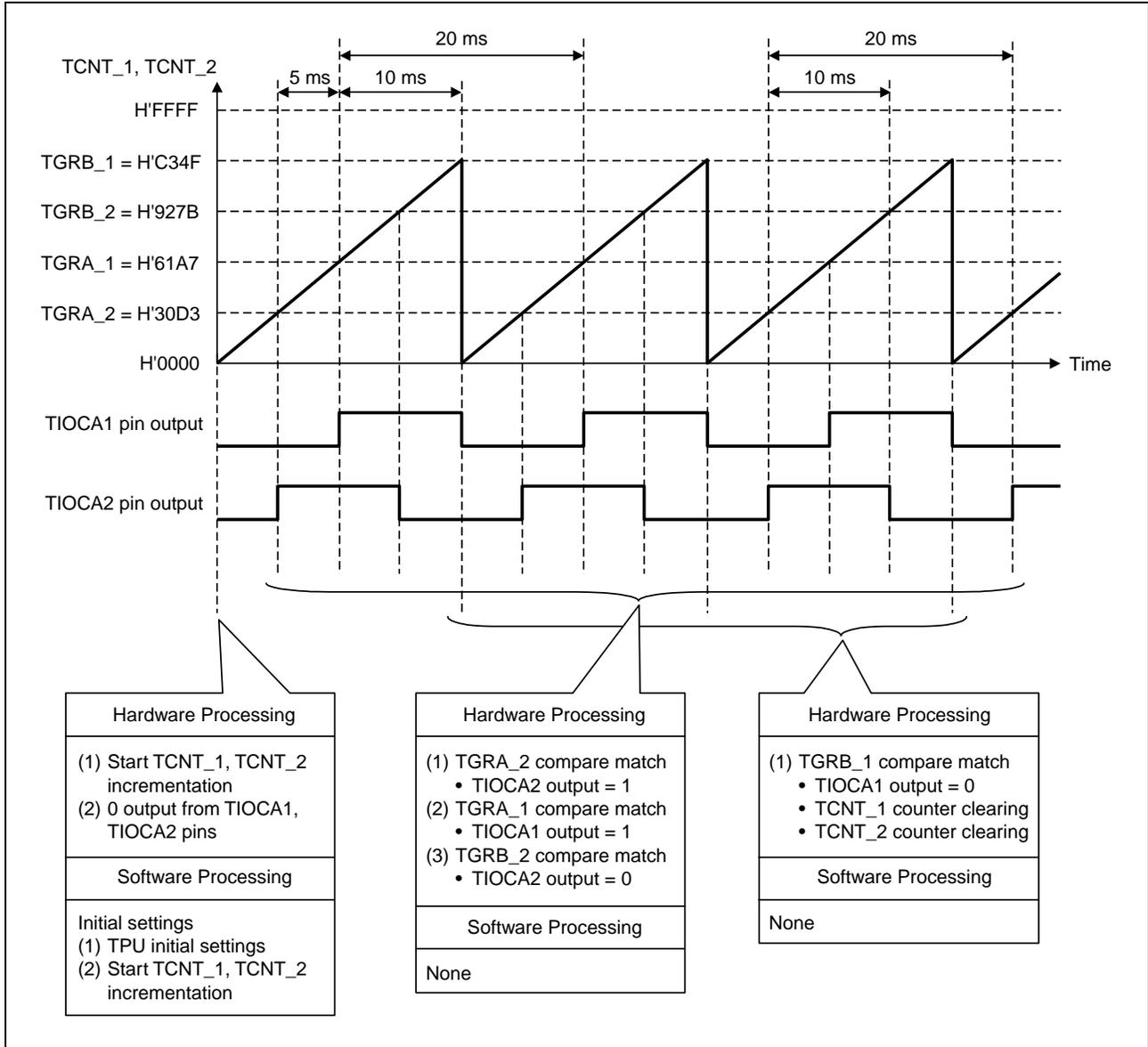
Figure 3 Principles of Operation
