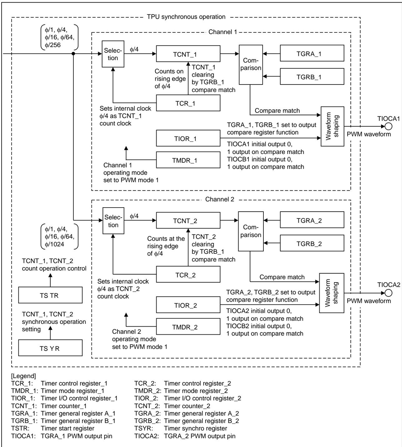
Figure 2 Block Diagram of TPU Synchronous Operation Function
