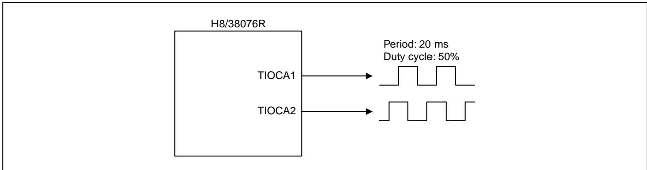
**Figure 1 Example of PWM Output Using TPU Synchronous Operation Function**
