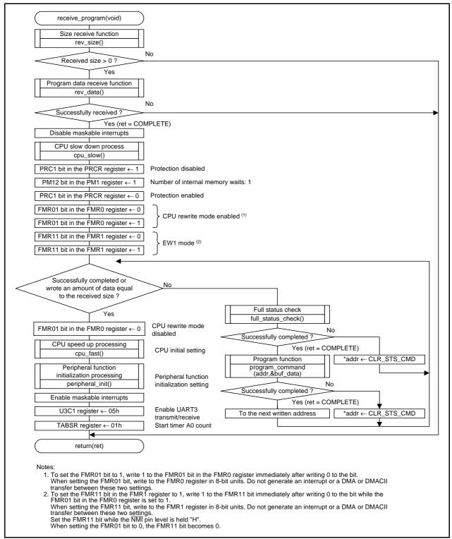
Figure 7.12 Flash Memory Write Function
