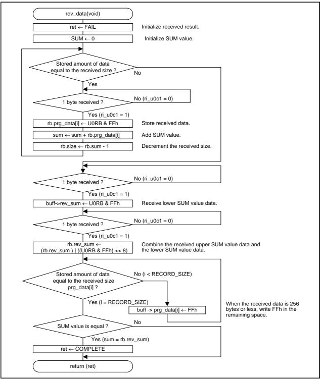
Figure 7.9 Program Data Receive Function
