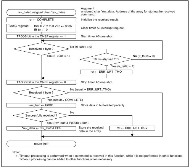
Figure 7.6 1-byte Command Receive Function
