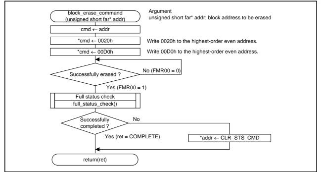
Figure 7.13 Block Erase Function
