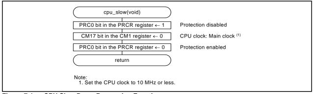
Figure 7.4 CPU Slow Down Processing Function
