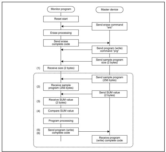
Figure 4.2 Monitor Program Operation Example
