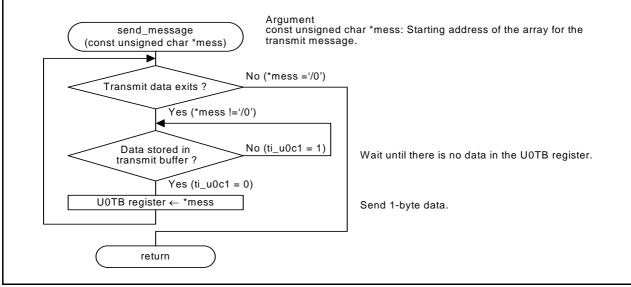
Figure 7.10 Message Transmit Function
