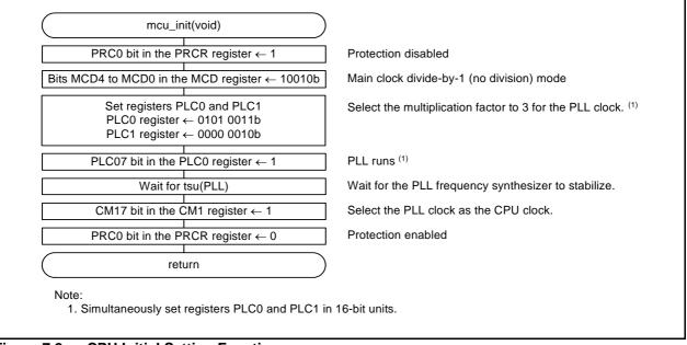
Figure 7.2 CPU Initial Setting Function
