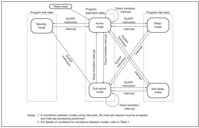
Figure 1 Mode transition diagram
