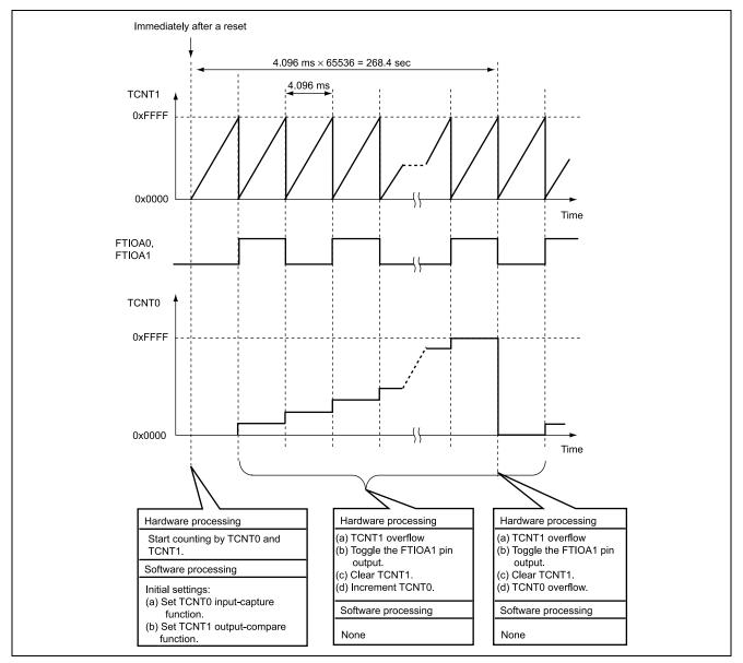
Figure 3.1 Principle of Operation
