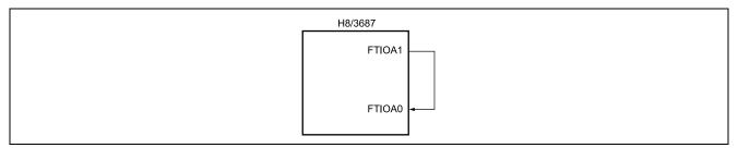
Figure 1.1 MPU Connection for Timer Z Cascade Operation
