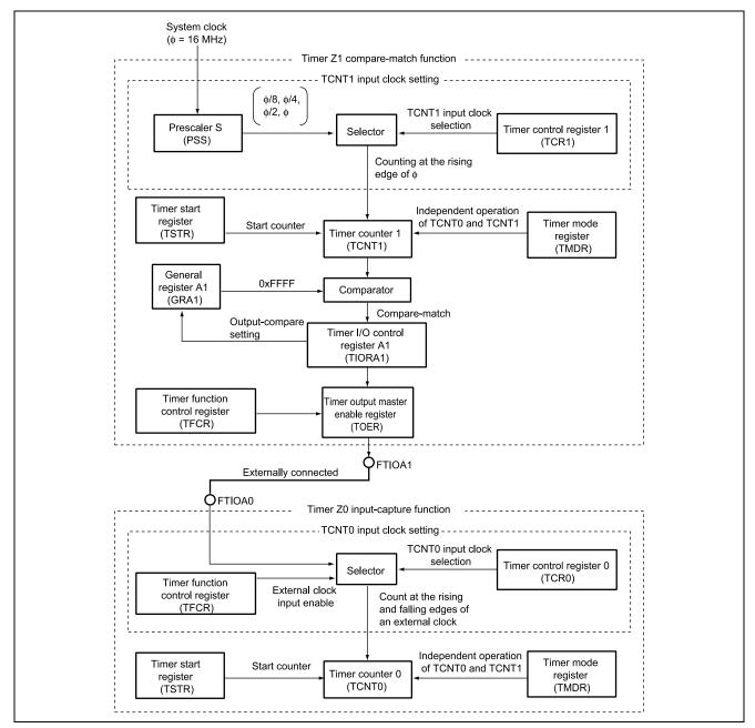
Figure 2.1 Block Diagram of the 32-bit Counter Using Timer Z Cascaded Connection
