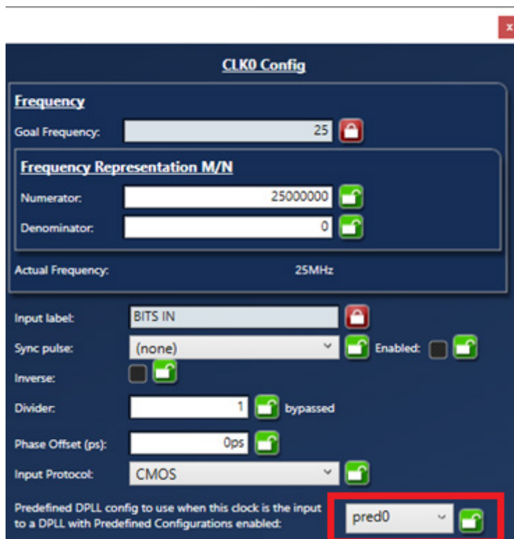
Figure 5. External Reference Configuration (clk0)
