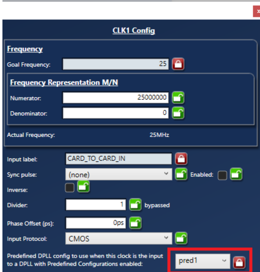
Figure 6. Card-to-Card Reference Configuration (clk1)
