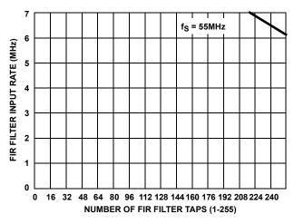
FIGURE 12A. THE NUMBER OF FILTER TAPS vs INPUT RATE FOR A DECIMATION OF 16
