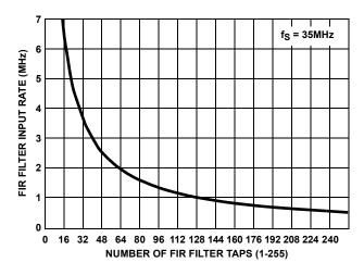
FIGURE 9. THE NUMBER OF FILTER TAPS vs INPUT RATE FOR A DECIMATION OF 2, SYM = 1, EVEN/ODD = 0
