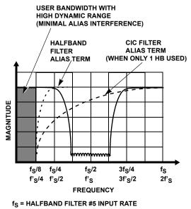
$f'_{S}$  = HALFBAND FILTER #5 OUTPUT RATE
