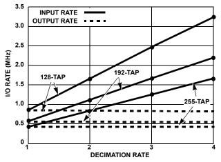
FIGURE 8A. DETERMINING MAXIMUM INPUT AND OUTPUT RATES, BASED ON FILTER DECIMATION FOR A 127, 192 AND 255 TAP FILTER (f<sub>S</sub> = 55MHz, SYM = 1, EVEN/ODD = 0)
