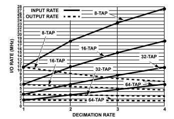
FIGURE 7A. DETERMINING MAXIMUM INPUT AND OUTPUT RATES BASED ON FILTER DECIMATION FOR A 8, 16, 32 AND 64 TAP FILTER (f<sub>S</sub> = 55MHz, SYM = 1, EVEN/ODD = 0)
