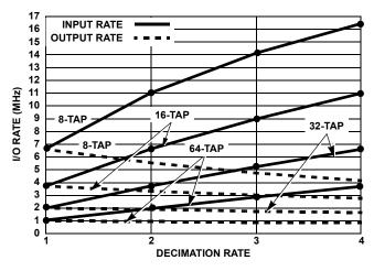
FIGURE 7. DETERMINING MAXIMUM INPUT AND OUTPUT RATES BASED ON FILTER DECIMATION FOR A 8, 16, 32 AND 64 TAP FILTER (f<sub>S</sub> = 33MHz, SYM = 1, EVEN/ODD = 0)
