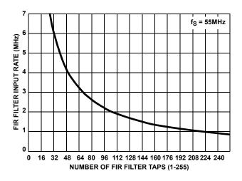
FIGURE 9A. THE NUMBER OF FILTER TAPS vs INPUT RATE FOR A DECIMATION OF 2, SYM = 1, EVEN/ODD = 0
