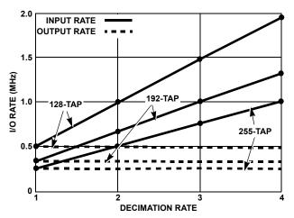
FIGURE 8. DETERMINING MAXIMUM INPUT AND OUTPUT RATES, BASED ON FILTER DECIMATION FOR A 127, 192 AND 255 TAP FILTER ( $f_S$  = 33MHz, SYM = 1, EVEN/ODD = 0)
