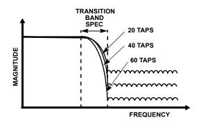
FIGURE 4C. FIXED TRANSITION BAND, VARIABLE OUT OF BAND REJECTION, VARIABLE NUMBER OF FILTER TAPS
