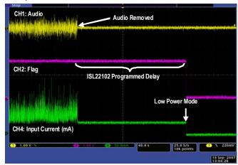
FIGURE 3. LOW POWER MODE WITH ISL22102
