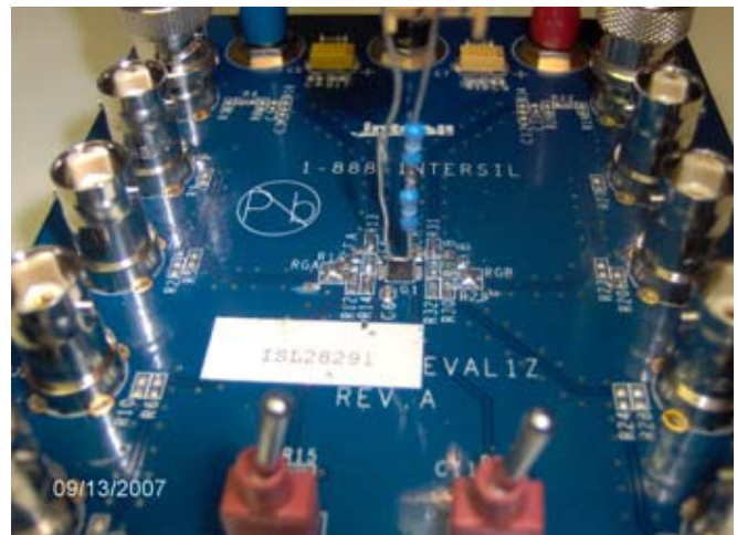
FIGURE 8. IMPROVED ANTENNA DESIGN TO EVALUATE RADIATED INTERFERENCE
