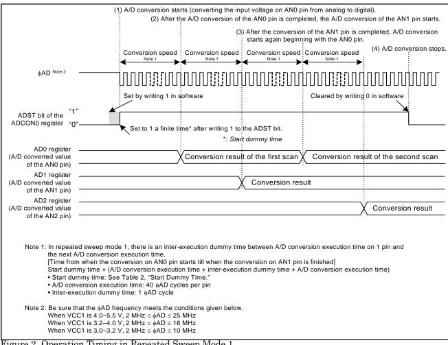
Figure 2. Operation Timing in Repeated Sweep Mode 1
