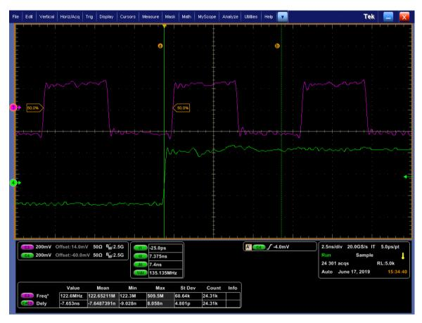
Figure 2. Sysref to QCLK Delay after Updating Sysref Global Phase Delay
