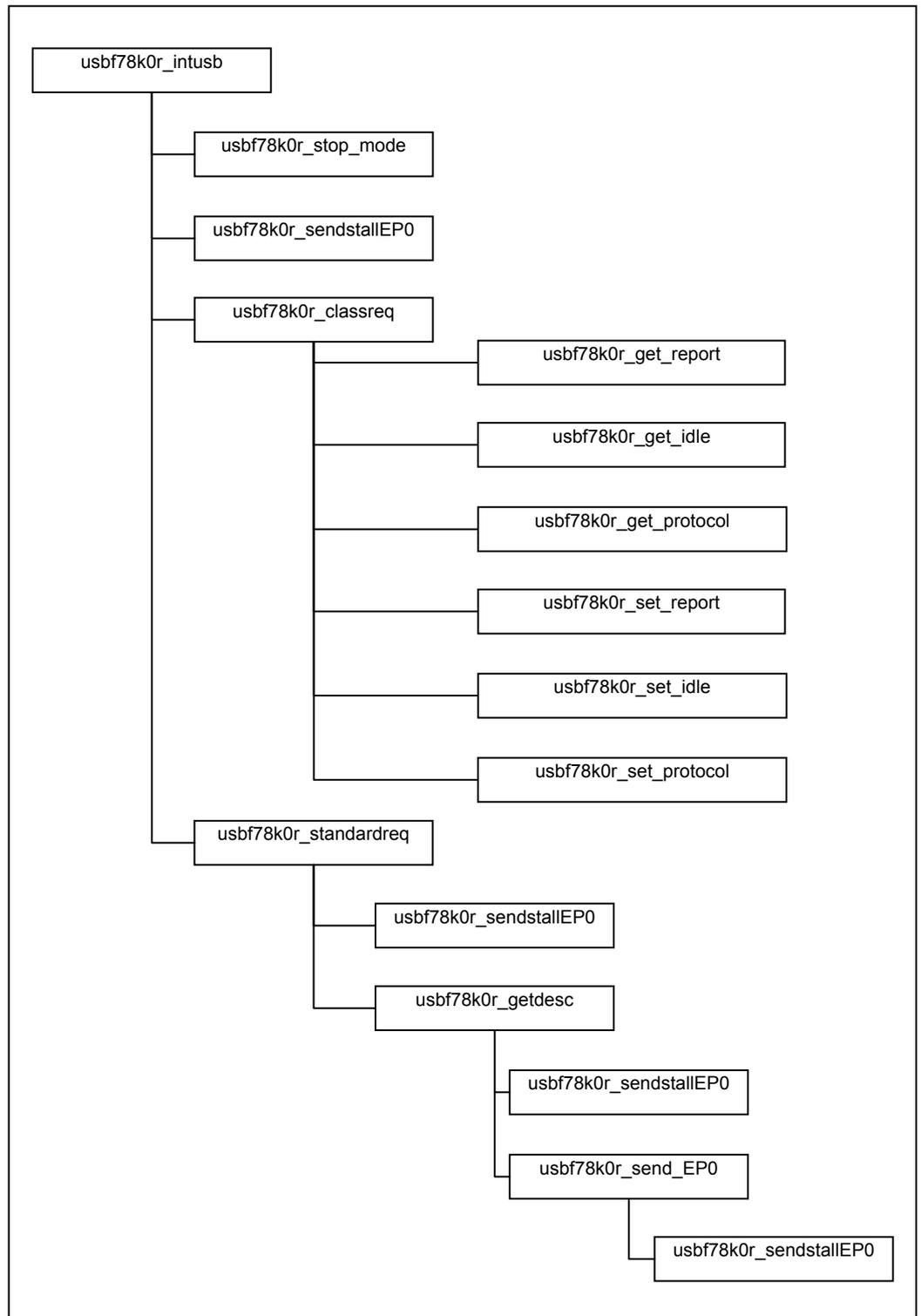
Figure 3-8 Calling Functions during the Processing for the USB HID Class (1)
