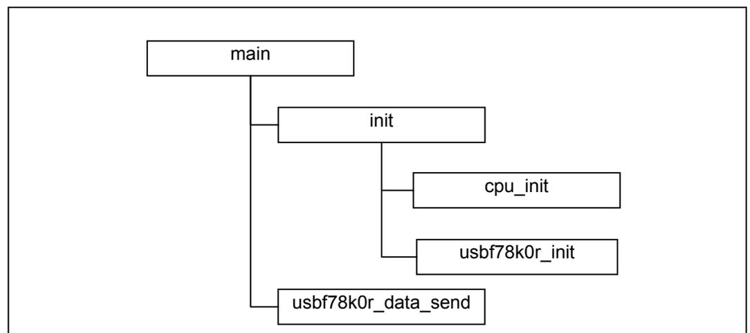
Figure 3-7 Calling Functions during the Processing for the USB function controller
