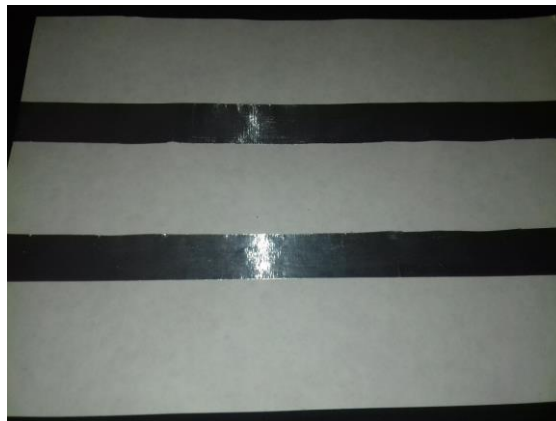
Figure 2. Resistive touch sensor built with metal foil
