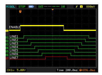
Figure 4. Linear Sequencer Functionality Waveform
