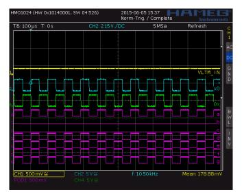
1. 90 mV on ADC input ('0' and '9' are displayed) 2. 180 mV on ADC input ('1' and '8' are displayed)
