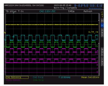
5. 450 mV on ADC input ('4' and '5' are displayed) 6. 540 mV on ADC input ('5' and '4' are displayed)
