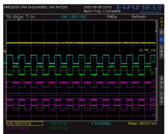
3. 270 mV on ADC input ('2' and '7' are displayed) 4. 360 mV on ADC input ('3' and '6' are displayed)
