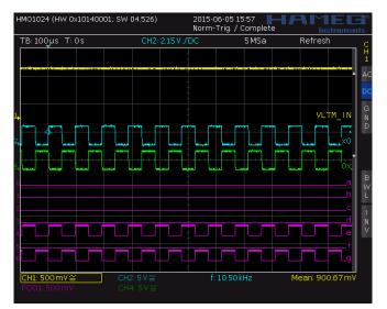
9. 810 mV on ADC input ('8' and '1' are displayed) 10. 900 mV on ADC input ('9' and '0' are displayed)
