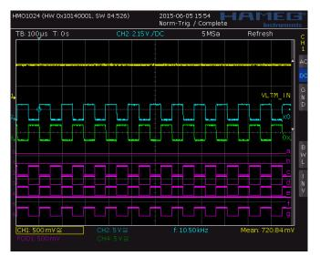
7. 630 mV on ADC input ('6' and '3' are displayed) 8. 720 mV on ADC input ('7' and '2' are displayed)
