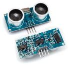
Fig 1. HC-SR04 Ultrasonic Sensor
