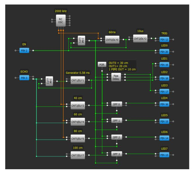
Fig 3. Ultrasonic Rangefinder schematic
