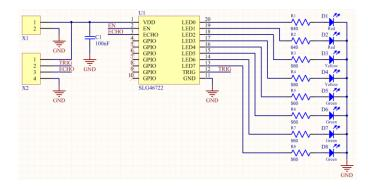
Fig 2. Ultrasonic Rangefinder typical application circuit
