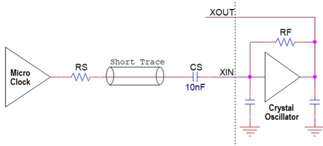
Keep the trace from the device output to crystal oscillator input pin as short as possible to minimize trace parasitic capacitance. When the trace is shorter than about 1 inch or 2.5cm, there is no need to design the trace as a transmission line and RS will not be needed. When designing the clock trace as a 50Ω transmission line, the proper value for RS is 22Ω to match the device output to the trace impedance.
