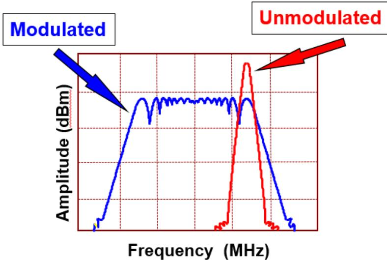
When the clock is not modulated, the frequency spectrum consists of harmonics that are narrow, like the red curve in Figure 6. Adding spread spectrum modulation, widens the peak at every harmonic, like the blue curve in Figure 6. Because each peak has a specific power level, making the peak wider also makes it less high. Adding spread spectrum to a clock lowers the ability of the clock to cause EMI.
