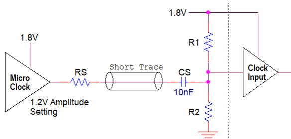
Use R1 = R2 to re-center the clock waveform at 50% of V<sub>DD</sub> = 1.8V. A good value for R1 = R2 is 100kΩ for 1MHz and higher clock frequencies. It is not recommended to use this method for 32.768kHz. The additional DC bias in R1 and R2 will be more than the supply current savings at the device output driver. For 32.768kHz, it is recommended to use the circuit in [Figure 3](#) and set the amplitude to what the clock input requires.
