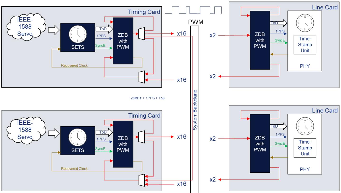
In AN-1033, there were several feedback paths for the RTT delay method introduced to the above diagram. In addition, most wireless infrastructure nodes also support transport of a recovered clock from each line card to each of the redundant pair of timing cards. This allows any line card to be the source of the master clock, which is traceable to the master time source in the network. This recovered clock is often a SyncE clock representing the exact desired frequency reference.
