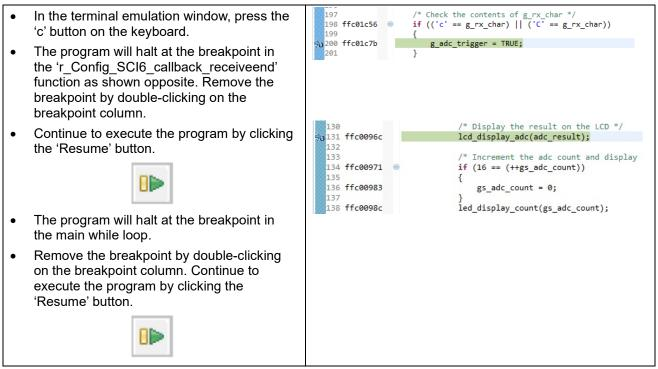
The program proceeds to display the result of the A/D conversion on the LCD and in the terminal window. In addition, the running count of A/D conversions performed is displayed in binary form using LEDs 0-3 on the RSK+. Adjust the potentiometer and press SW1, SW2 or SW3 on the RSK+ and an additional A/D conversion will be performed.
