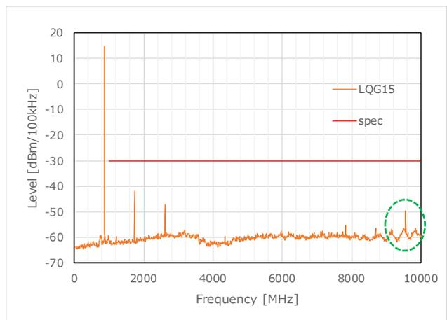
Figure 11 TX Harmonics\_LQG15 (869.3MHz)
