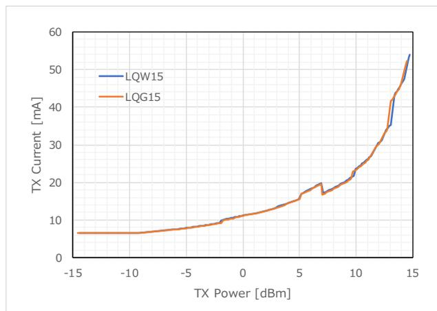
Figure 59 TX Current (915.0MHz)
