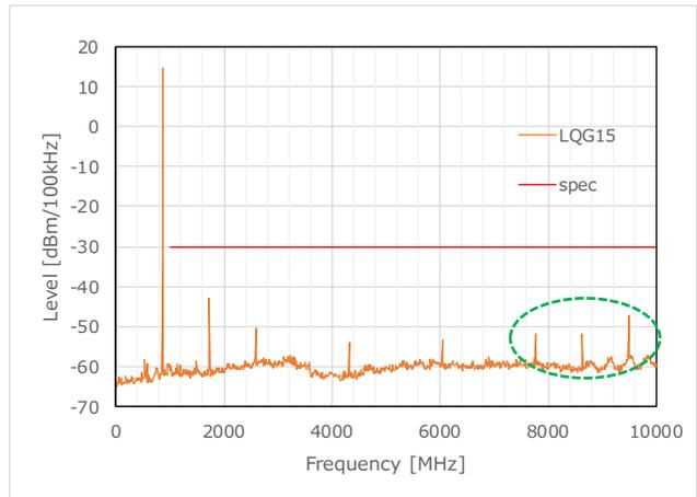
Figure 45 TX Harmonics\_LQG15 (863.1MHz)
