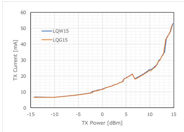
Figure 3 TX Current (863.1MHz)
