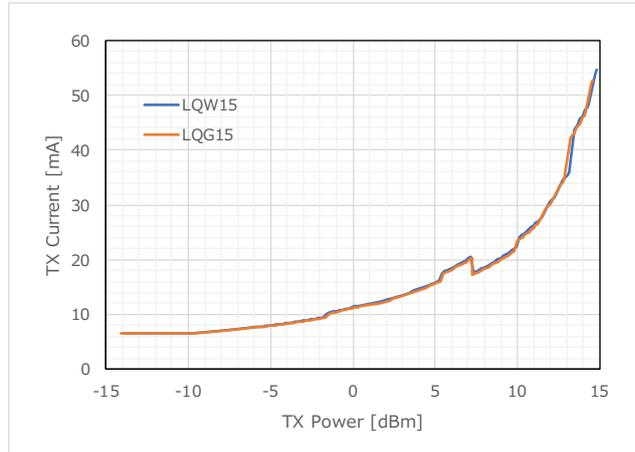
Figure 21 TX Current (902.2MHz)
