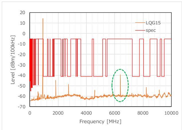
Figure 65 TX Harmonics\_LQG15 (915.0MHz)
