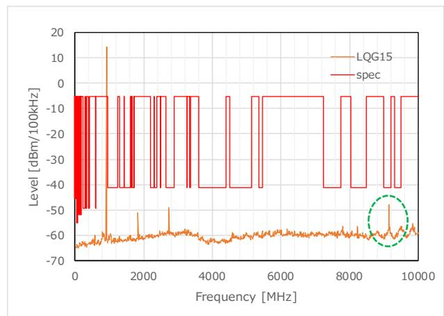
Figure 29 TX Harmonics\_LQG15 (915.0MHz)
