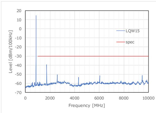
Figure 44 TX Harmonics\_LQW15 (863.1MHz)
