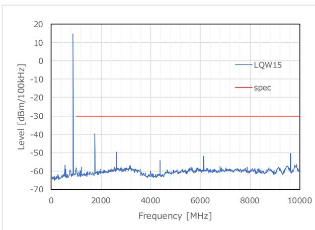
Figure 48 TX Harmonics\_LQW15 (875.5MHz)
