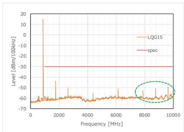
Figure 49 TX Harmonics\_LQG15 (875.5MHz)
