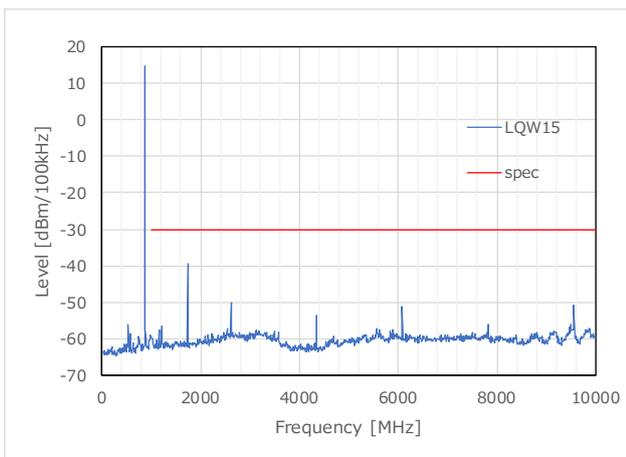
Figure 46 TX Harmonics\_LQW15 (869.3MHz)
