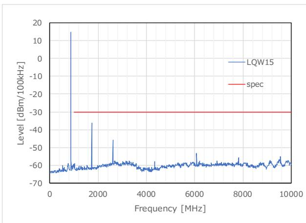
Figure 10 TX Harmonics\_LQW15 (869.3MHz)
