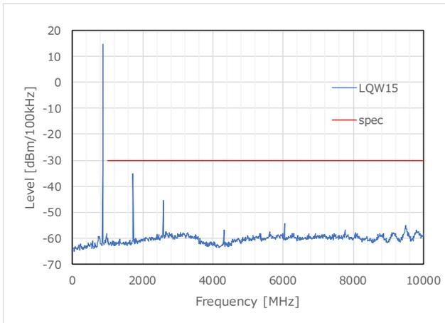
Figure 8 TX Harmonics\_LQW15 (863.1MHz)
