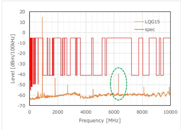
Figure 63 TX Harmonics\_LQG15 (902.2MHz)
