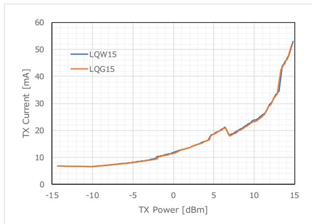
Figure 5 TX Current (869.3MHz)
