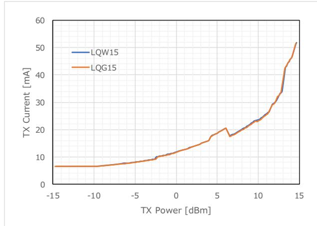
Figure 39 TX Current (863.1MHz)
