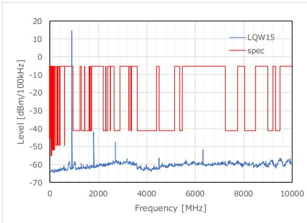
Figure 26 TX Harmonics\_LQW15 (902.2MHz)
