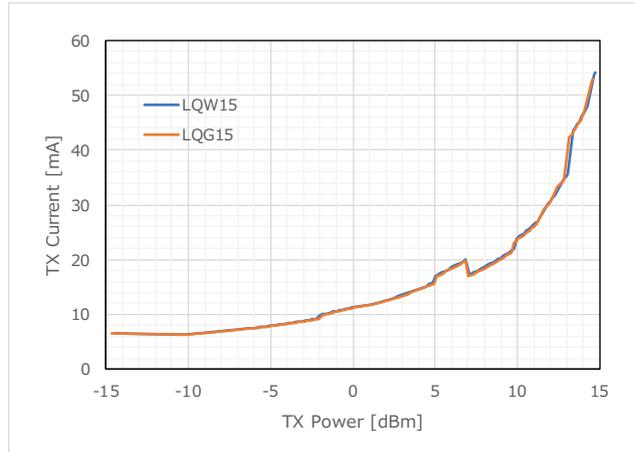
Figure 57 TX Current (902.2MHz)
