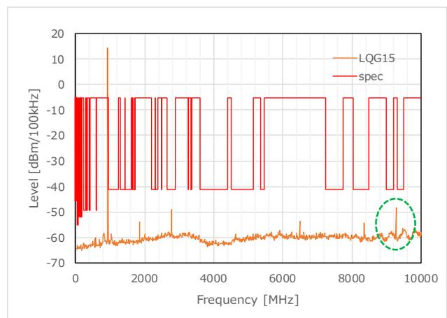
Figure 31 TX Harmonics\_LQG15 (927.8MHz)
