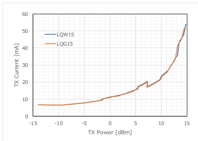
Figure 23 TX Current (915.0MHz)
