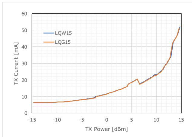
Figure 43 TX Current (875.5MHz)
