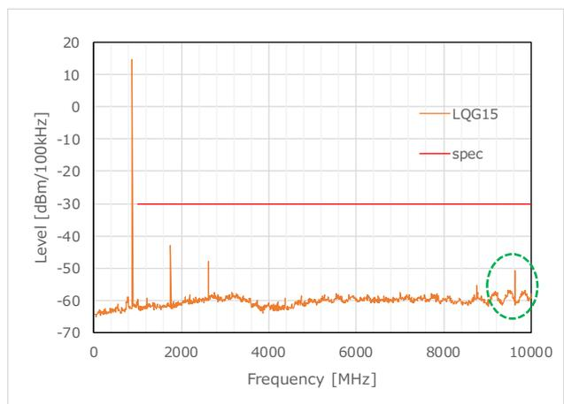
Figure 13 TX Harmonics\_LQG15 (875.5MHz)
