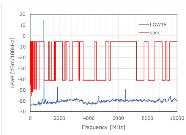
Figure 30 TX Harmonics\_LQW15 (927.8MHz)
