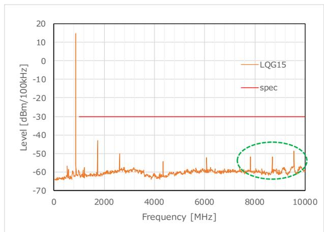
Figure 47 TX Harmonics\_LQG15 (869.3MHz)
