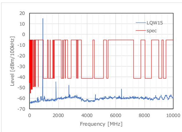
Figure 28 TX Harmonics\_LQW15 (915.0MHz)
