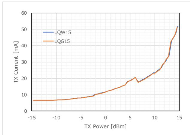
Figure 41 TX Current (869.3MHz)
