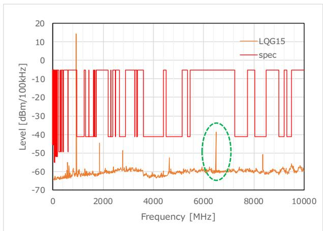
Figure 67 TX Harmonics\_LQG15 (927.8MHz)
