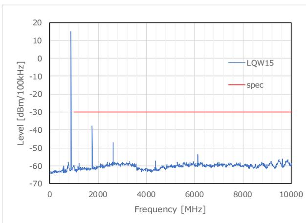
Figure 12 TX Harmonics\_LQW15 (875.5MHz)
