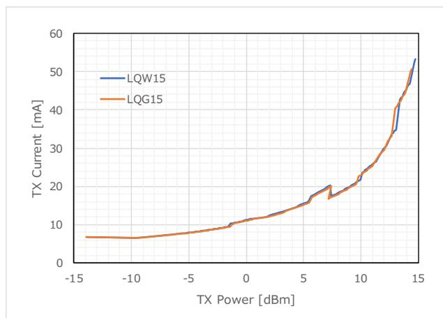
Figure 25 TX Current (927.8MHz)
