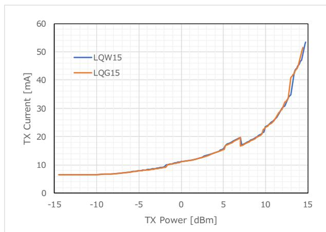
Figure 61 TX Current (927.8MHz)
