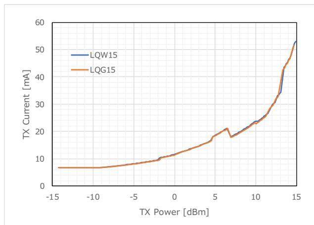
Figure 7 TX Current (875.5MHz)
