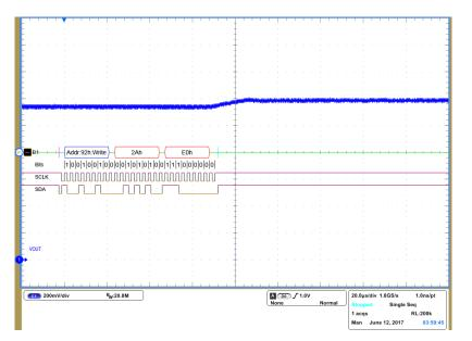
Figure 14: DVC Step-Up from 1.15 V to 1.2 V
