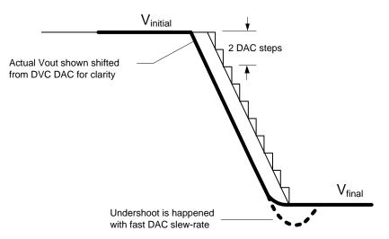
Figure 4: PV88080 DVC Down Transition Measurement Example
