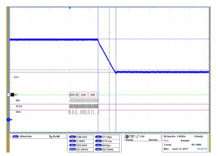
Figure 10: DVC Step-Down with 12.5 mV/µs Slew Rate
