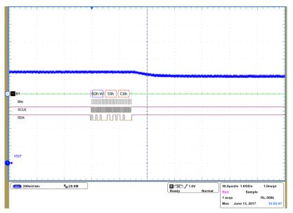
Figure 16: DVC Step-Down from 1.05 V to 1.0 V
