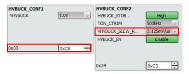
Figure 15: Sending 0xC8 to HVBUCK in Dialog GUI
