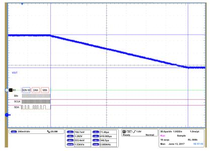
Figure 8: DVC Step-Down with 1.5625 mV/µs Slew Rate
