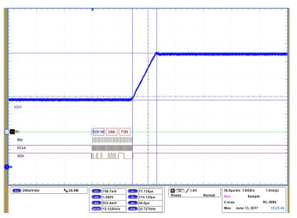
Figure 9: DVC Step-Up with 12.5 mV/µs Slew Rate
