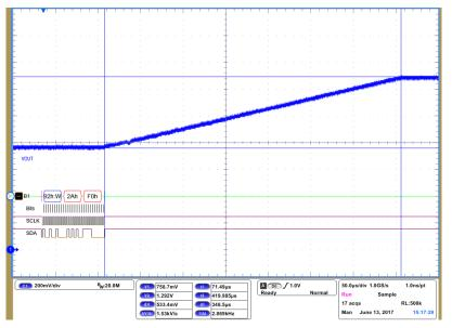
Figure 7: DVC Step-Up with 1.5625 mV/µs Slew Rate
