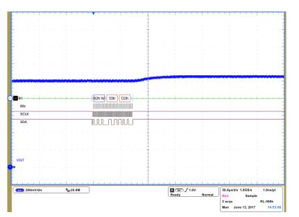
Figure 18: DVC Step-Up from 1.0 V to 1.05 V
