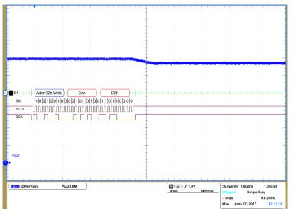
Figure 12: DVC Step-Down from 1.2 V to 1.15 V
