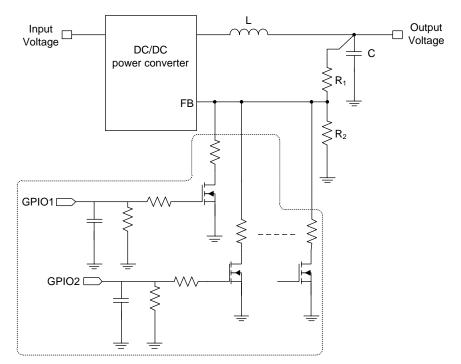
Figure 1: Traditional DVC Solution
