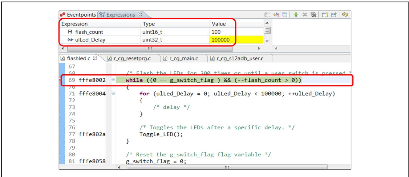
Figure 2-9 Execution of Event Break – Switch “SEQUENCE”
