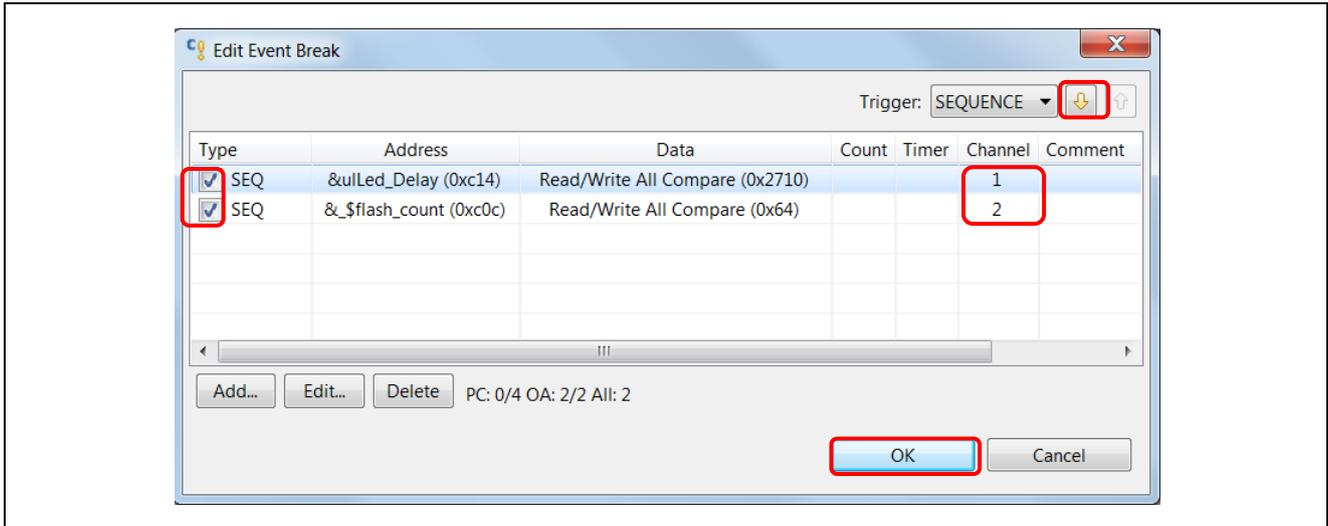
Figure 9 [Edit Event Break] - Switch Channel “SEQUENCE”
