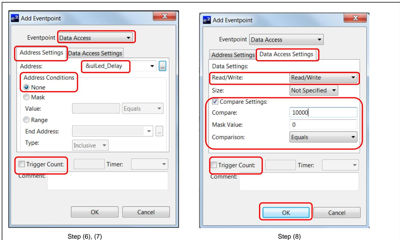
**Figure 4 [Add Eventpoint] Settings for global variable “Led\_Delay”**
