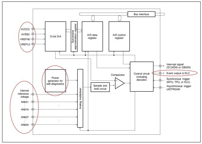
Figure 1.1 Block Diagram of 12-Bit A/D Converter of RX231 Group
