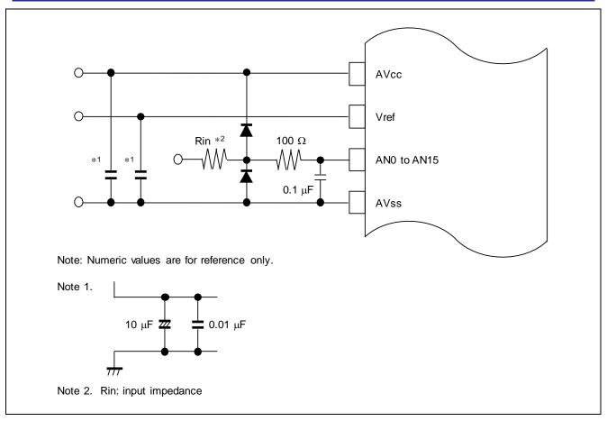
Figure 4.4 Example Analog Input Protection Circuit for H8S/2378 Group
