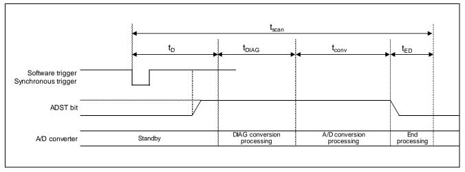
Figure 3.4 RX231 Group Scan Conversion Timing (Software Activation and Synchronous Trigger Activation)
