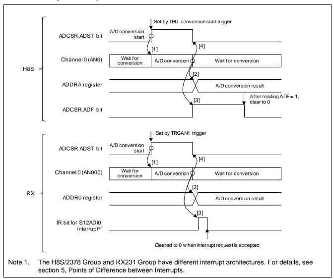
Figure 3.1 Single Mode Operation Timing Chart
