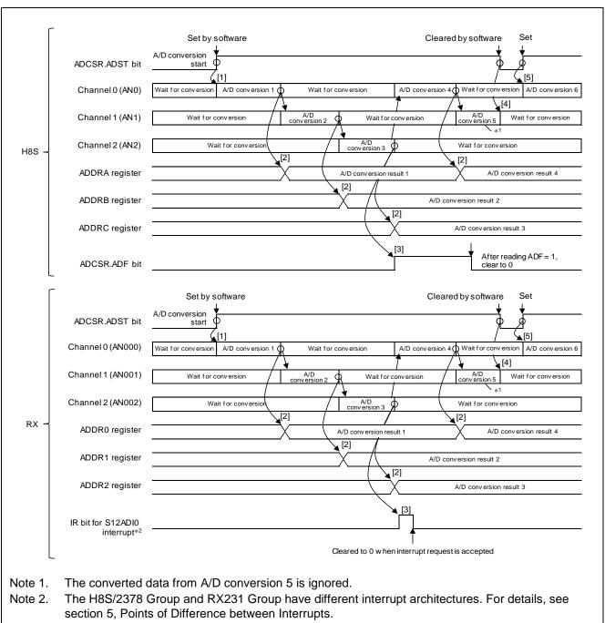
Figure 3.2 Scan Mode Operation Timing Chart
