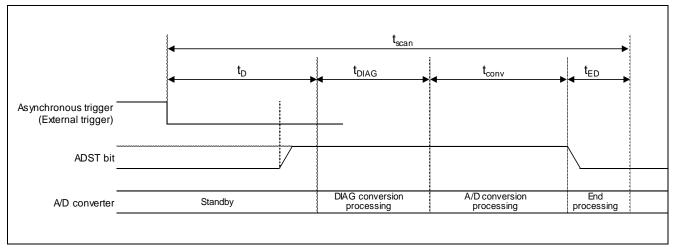
Figure 3.5 RX231 Group Scan Conversion Timing (Asynchronous Trigger Activation)
