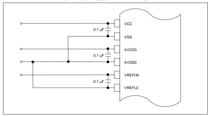
Figure 4.2 Connection Example of RX231 Group Power Supply Pins
