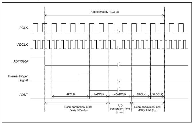
Figure 3.6 Timing Chart of Asynchronous Trigger Input to A/D Conversion End on RX231 Group
