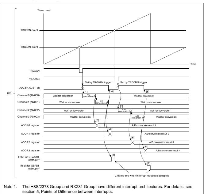
Figure 3.3 Group Scan Mode Operation Timing Chart
