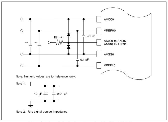
Figure 4.3 Example Analog Input Protection Circuit for RX231 Group
