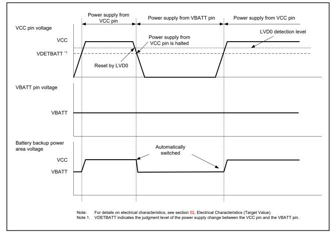
Figure 12.2 Operation for Switching to Battery Backup Function
