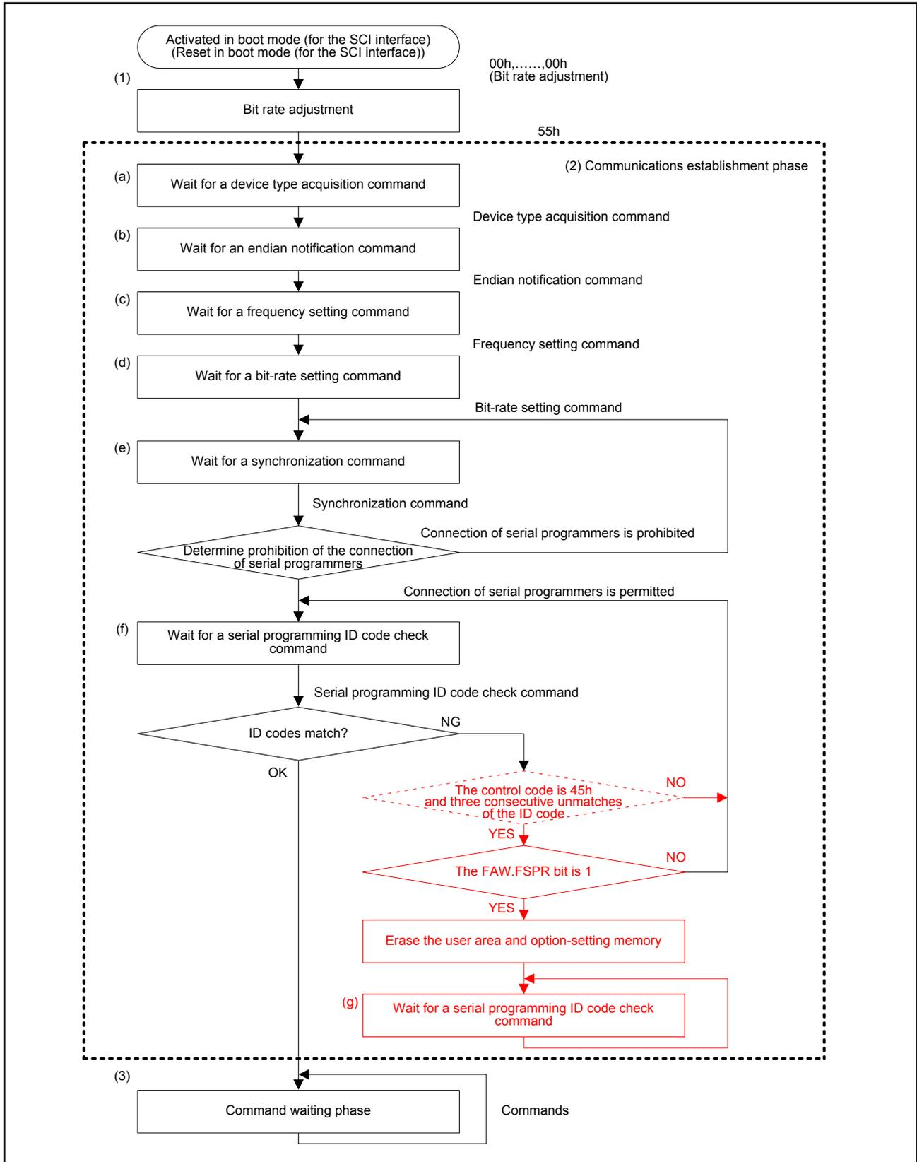
Figure 56.8 State Transition Flow in Boot Mode (for the SCI Interface)
