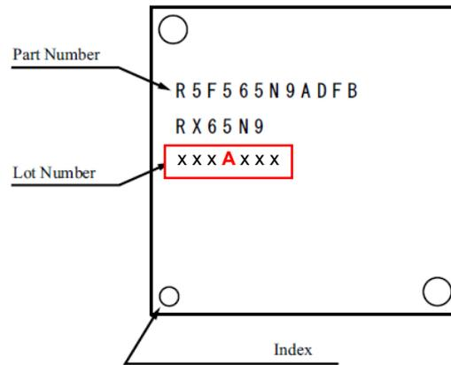
Note 1. The above figure is an example of mark specification.
