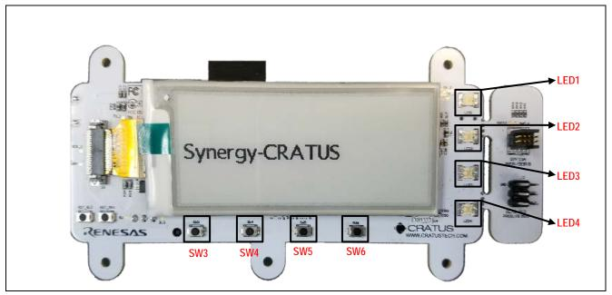
Figure 1 ITMM Reference Solution Board
