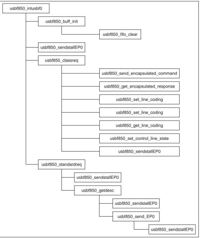
Figure 4.7 Function Calls in USB Function Control Processing
