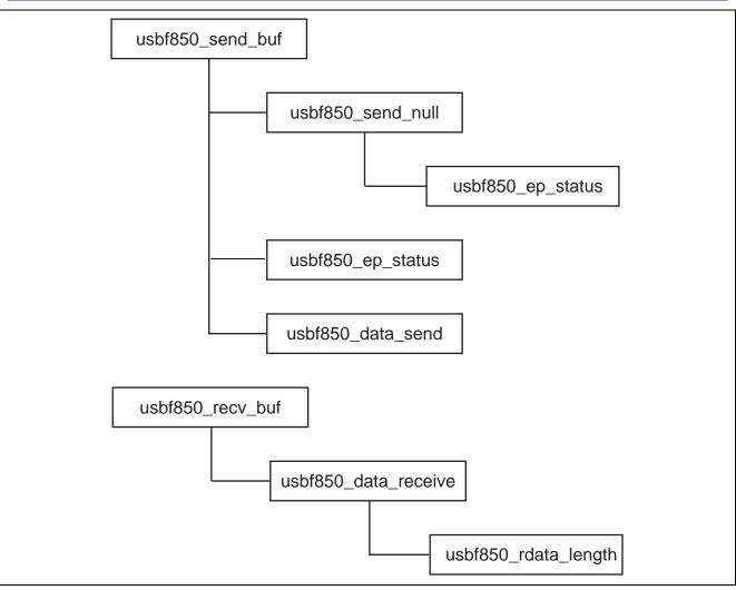
Figure 4.9 Function Calls in USB Communication Class Processing (2/2)
