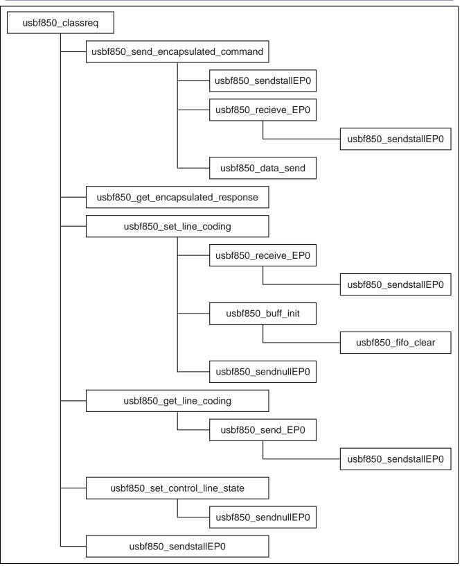
Figure 4.8 Function Calls in USB Communication Class Processing (1/2)
