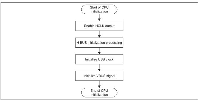
Figure 4.2 CPU Initialization Processing Flow
