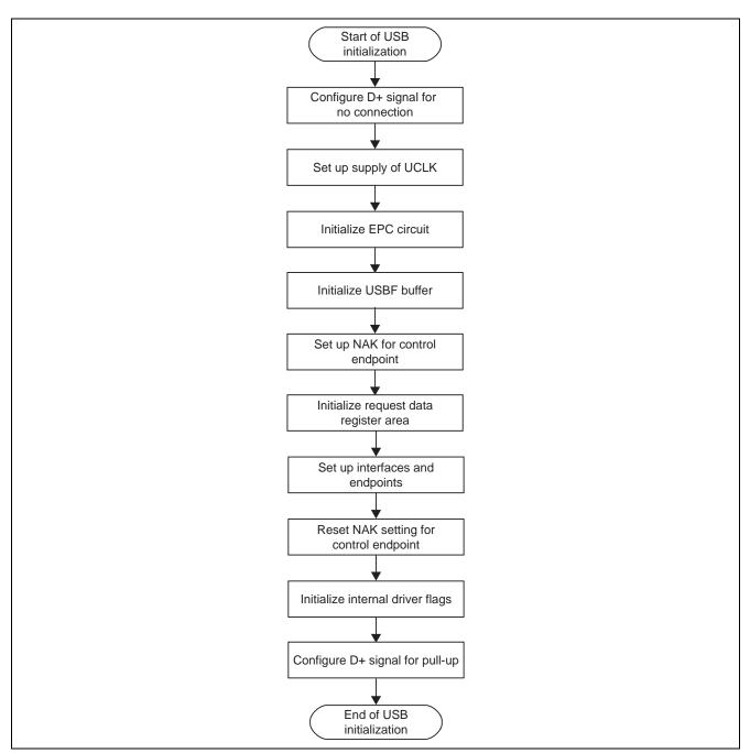
Figure 4.3 USB Function Controller Initialization Processing Flow
