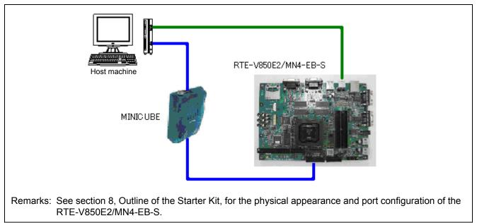
Figure 6.1 System Configuration of the Development Environment
