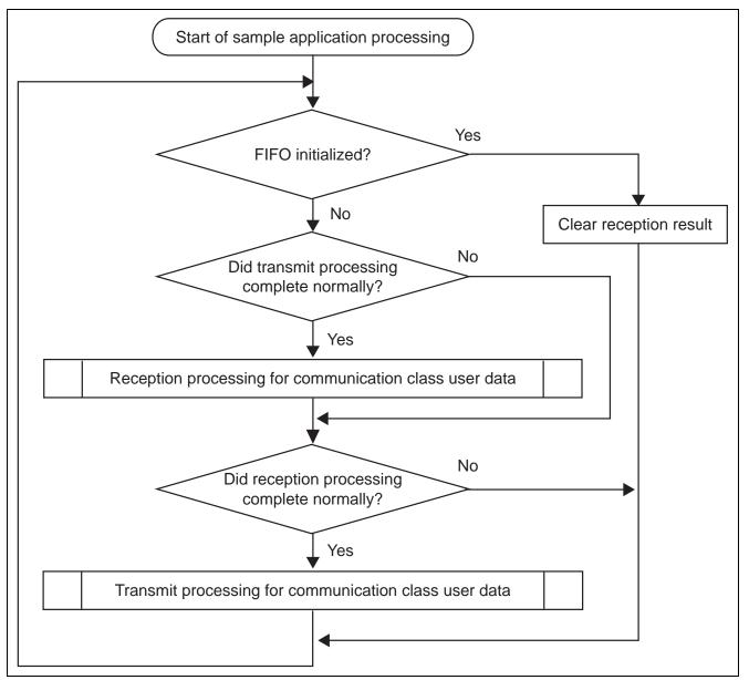
Figure 5.1 Sample Application Processing Flowchart
