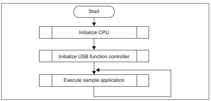
Figure 4.1 Sample Driver Processing Flow
