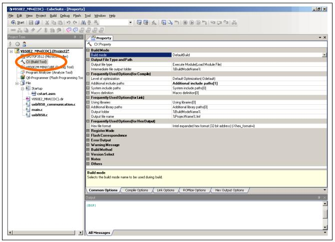
Figure 6.6 Selecting the Build Tool
