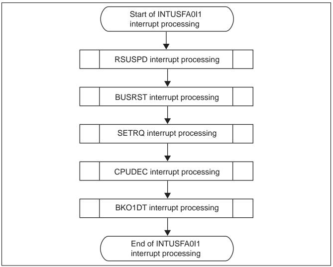
Figure 4.5 INTUSFA0I1 Interrupt Handler Processing Flow
