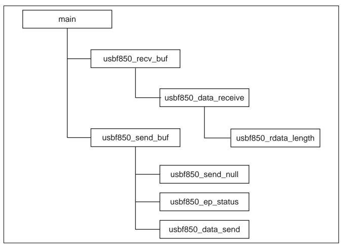
Figure 4.6 Function Calls within main Processing
