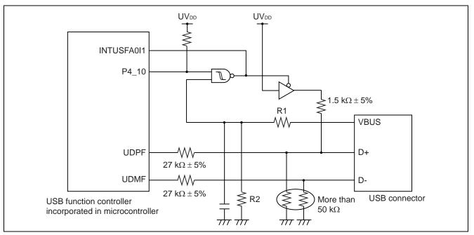
Figure 4.4 USB Function Controller Configuration Example
