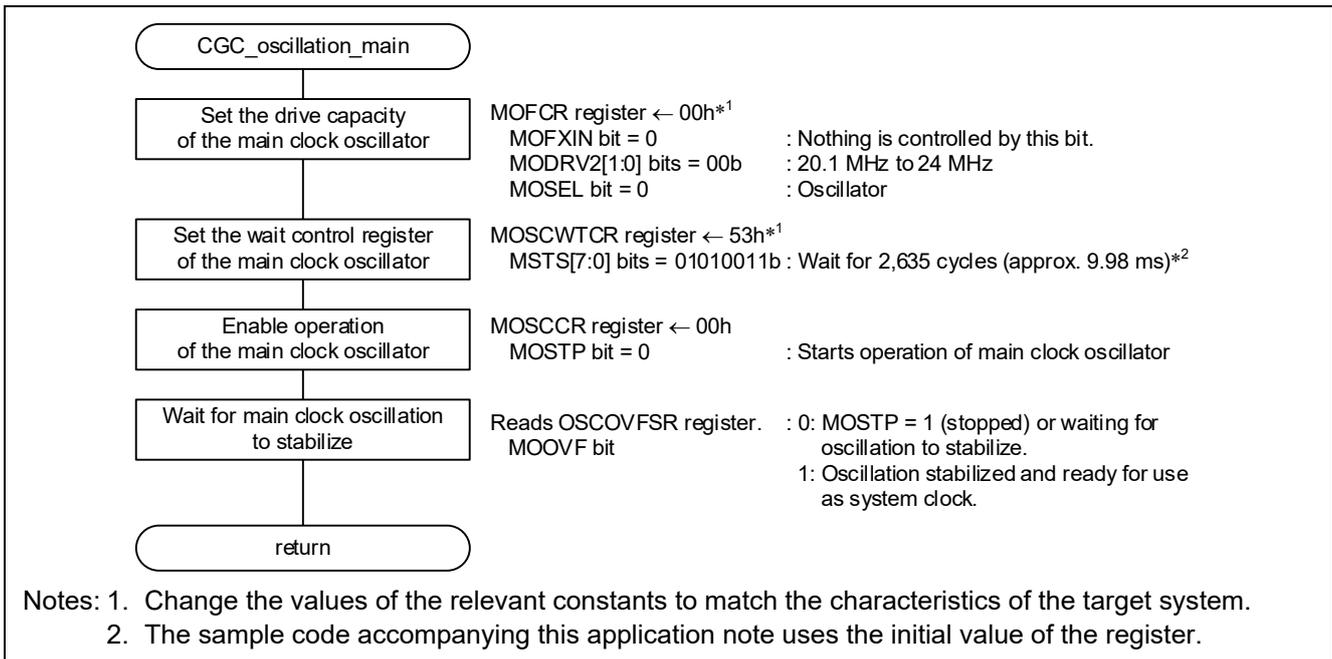
Figure 3.6 Main Clock Oscillation Enable
