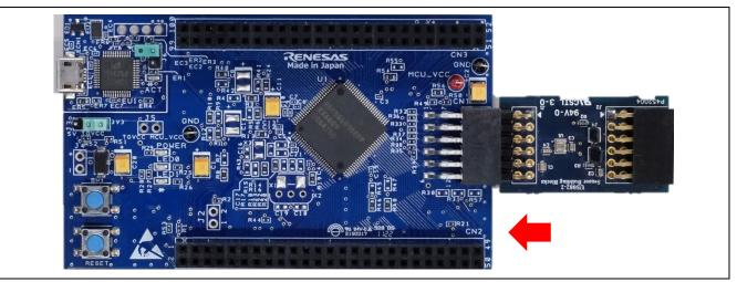
Figure 6-7 Connecting the Sensor Board to the Pmod Connector on the TB-RX660
