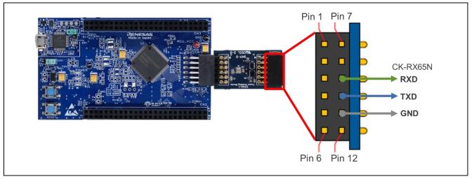
Figure 6-8 Locations of Pins on the TB-RX660 Used for UART Communications between the Microcontrollers
