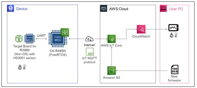
Figure 3-1 System Configuration of This Demo
