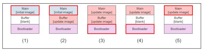
Figure 4-3 States of ROM in the Secondary MCU during Updating
