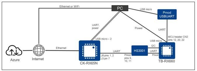
Figure 6-1 Overall Hardware Structure for This Demo
