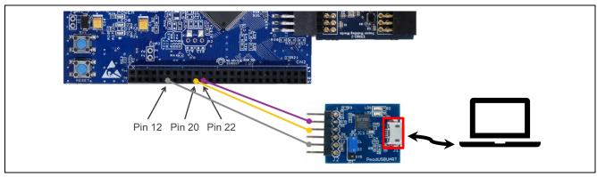
Figure 6-9 Connecting TB-RX660 with the Serial Communications Cable for Log Output to the PC
