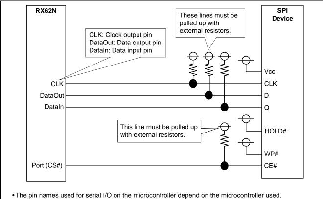
In this application note, the pins used are expressed as the CLK, DataIn, DataOut, and Port (CS#) pins to match the notation used in the sample code.
