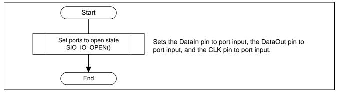
Figure 6.8 Serial I/O Open Setup Processing Outline
