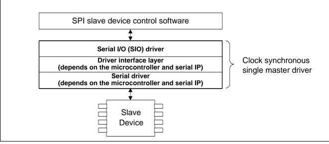
Figure 6.2 Software Structure
