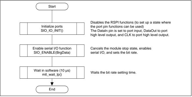
Figure 6.7 Serial I/O Enable Setup Processing Outline
