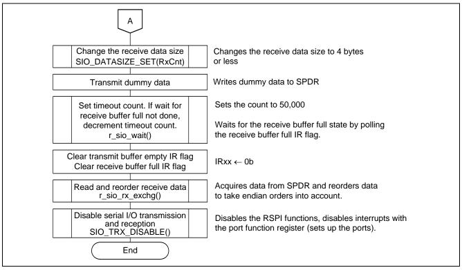
Figure 6.14 Serial I/O Data Reception Processing Outline — 4 (High-Speed Reception)
