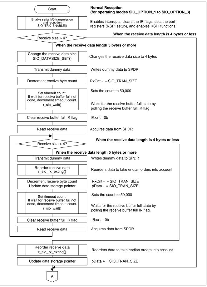
Figure 6.11 Serial I/O Data Reception Processing Outline — 1 (Normal Reception)
