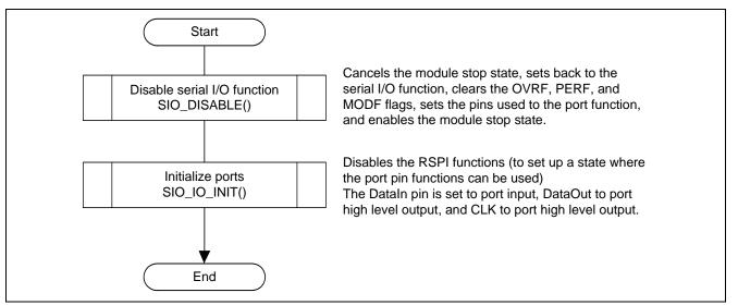
Figure 6.6 Serial I/O Disable Setup Processing Outline
