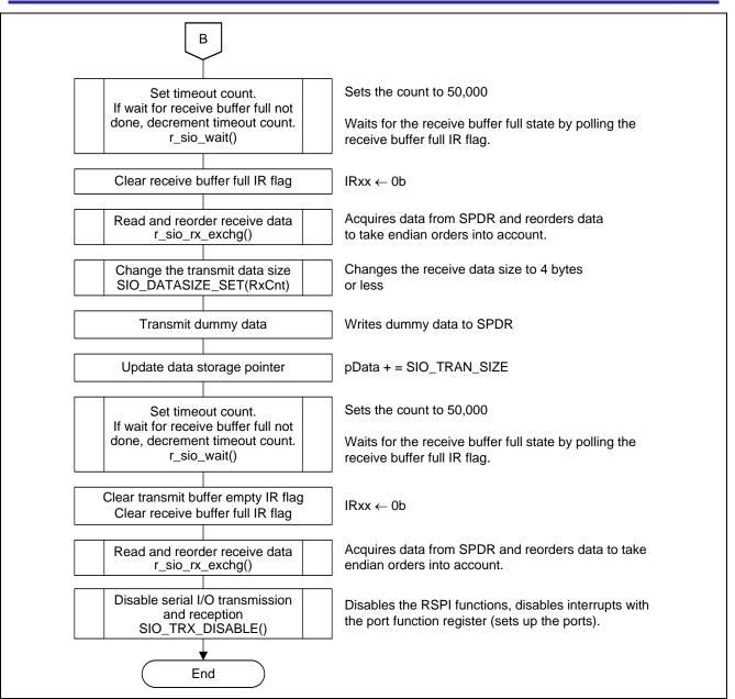
Figure 6.15 Serial I/O Data Reception Processing Outline — 5 (High-Speed Reception)
