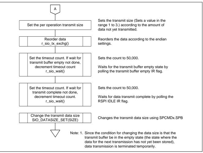
Figure 6.10 Serial I/O Data Transmission Processing Outline — 2
