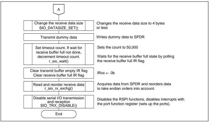
Figure 6.12 Serial I/O Data Reception Processing Outline — 2 (Normal Reception)
