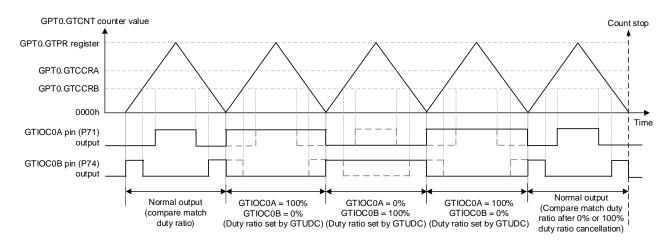
Figure 1.1 PWM Output Produced by rx24u\_gpt\_sample1
