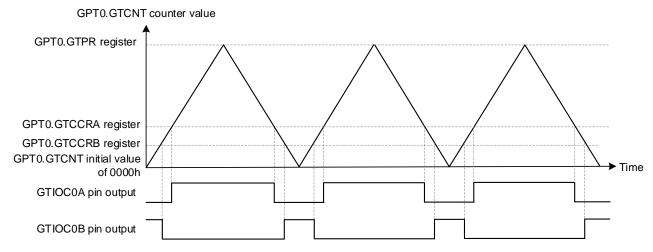
Figure 4.1 Triangle-Wave Complementary PWM Mode 1 Signal Generation Example (GTCCRA > GTCCRB)
