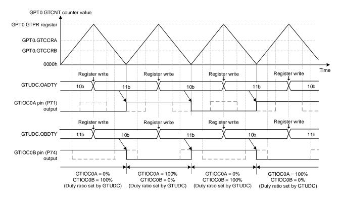
Figure 4.3 Example of Initial Duty Ratio (Count Stop) Setting and Its Reflection in Output after Count Operation Start
