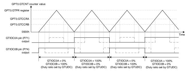
Figure 1.2 PWM Output Produced by rx24u\_gpt\_sample2
