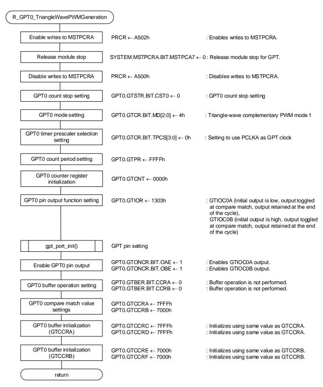
Figure 4.5 Triangle-Wave Complementary PWM Generation
