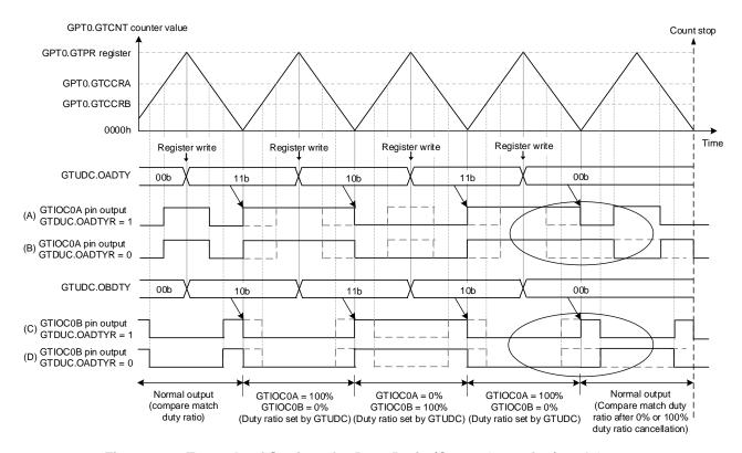
Figure 4.2 Example of Settings for Duty Ratio (Count Operation) and Output After Duty Ratio Cancellation
