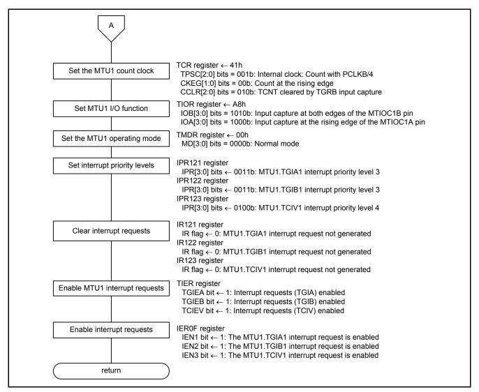
Figure 5.6 Peripheral Function Initialization (2/2)
