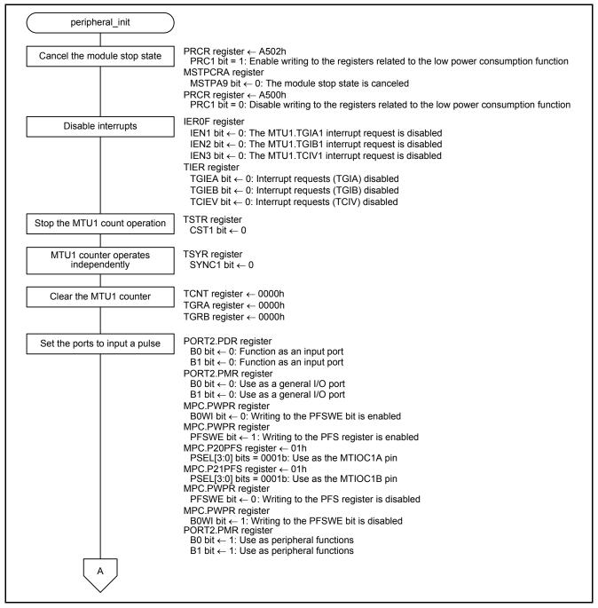
Figure 5.5 Peripheral Function Initialization (1/2)
