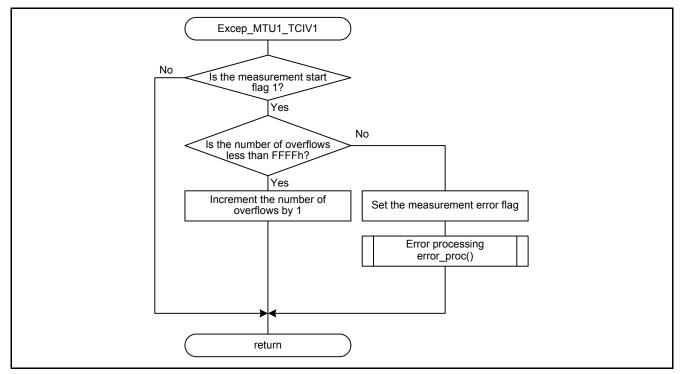
Figure 5.18 MTU1 Overflow Interrupt Handler
