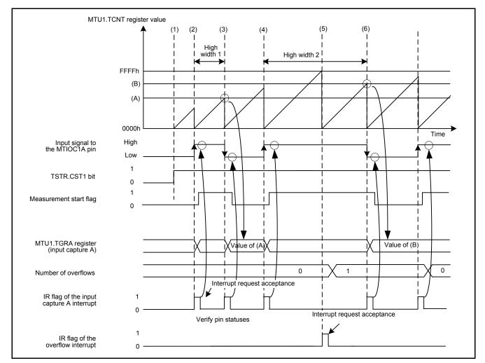
Figure 5.11 Timing Diagram of the Pulse Width Measurement
