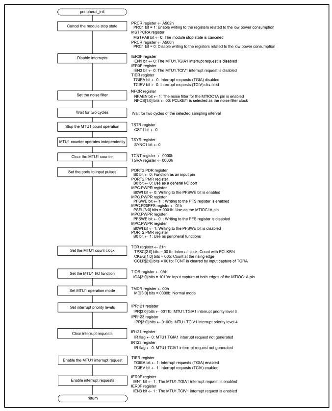
Figure 5.15 Peripheral Function Initialization
