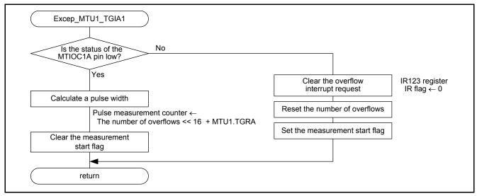
Figure 5.17 MTU1 Input Capture A Interrupt Handler
