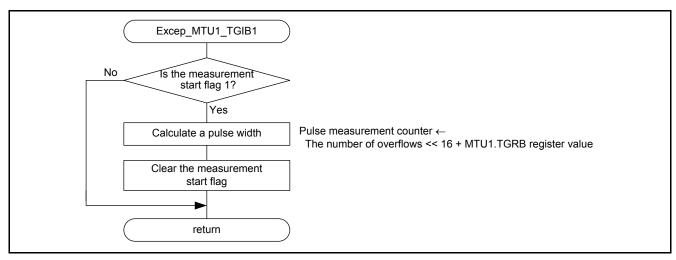
Figure 5.9 MTU1 Input Capture B Interrupt Handler
