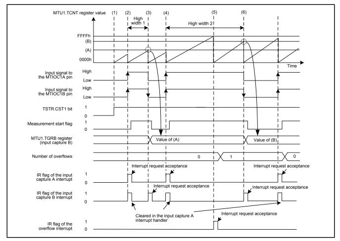
Figure 5.1 Timing Diagram of the Pulse Width Measurement
