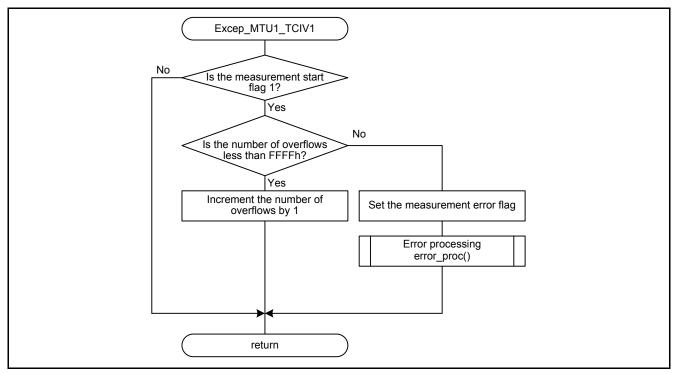
Figure 5.10 MTU1 Overflow Interrupt Handler
