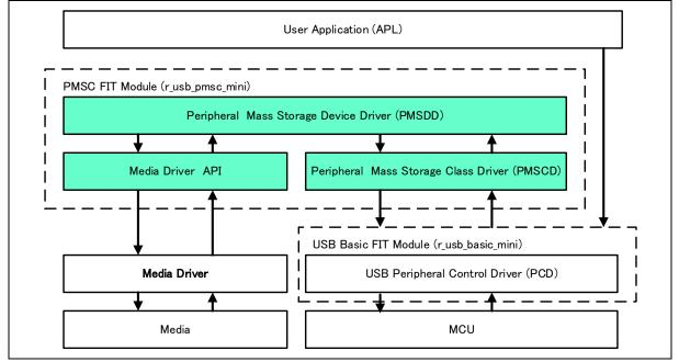
Figure 2-1 Software Module Structure
