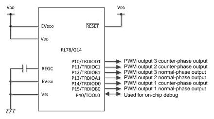
From G14 Application Note: Figure 3.1 Hardware Configuration
