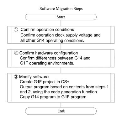
For a detailed example, refer to RL78/G14 Timer RD (Reset Synchronized PWM Mode) CC-RL (document R01AN2506EJ0100, referred to as RL78/G14 Application Note, herein). The Application Note explains how to modify the G1F program with the G14 program. RL78/G1F hardware is configured to support the RL78/G1F target board (YQB-R5F11BLE-TB) CPU board mounted on R5F11BLE.
