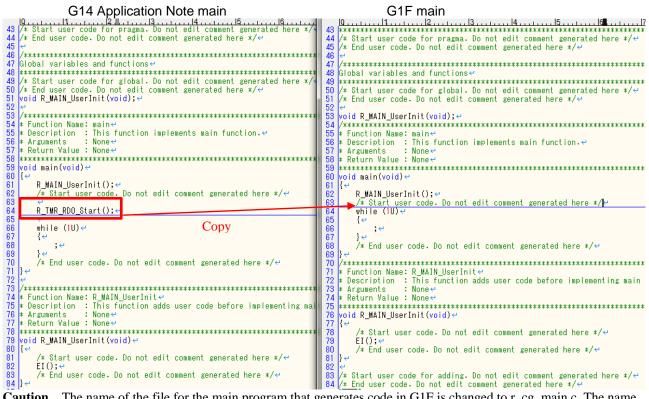
**Caution** The name of the file for the main program that generates code in G1F is changed to r\_cg\_main.c. The name of the R\_TMR\_RD0\_Start() function is also changed to R\_TMRD0\_Start() in G1F. The user will need to change file names accordingly.
