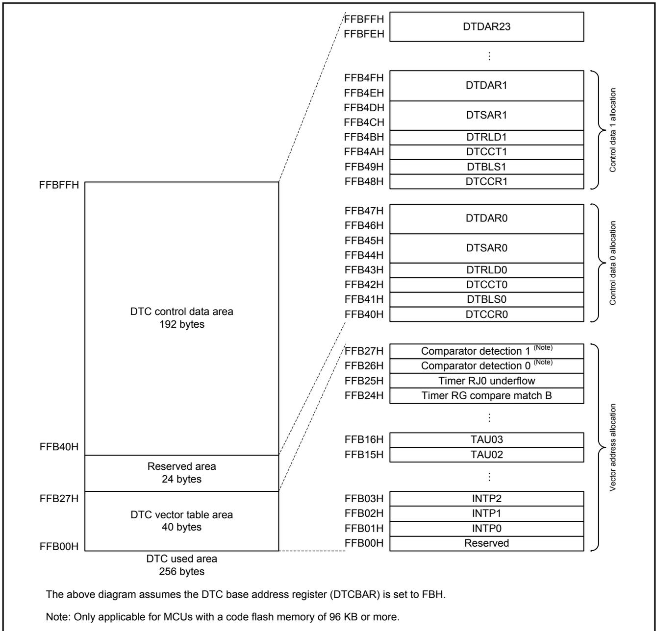
Figure 3.1 Memory Map When the DTCBAR Register is Set to FBH
