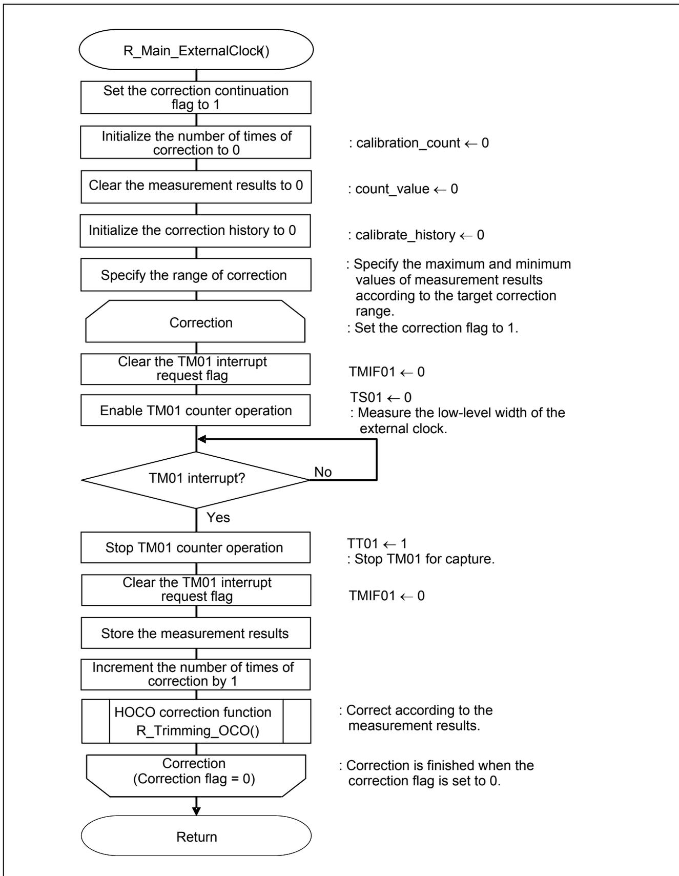
Figure 5.14 Calibration with External Input Clock
