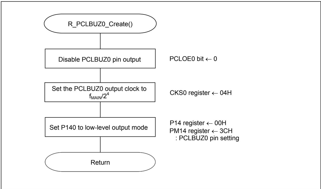
**Figure 5.8 Clock Output/Buzzer Output Control Circuit Setup**
