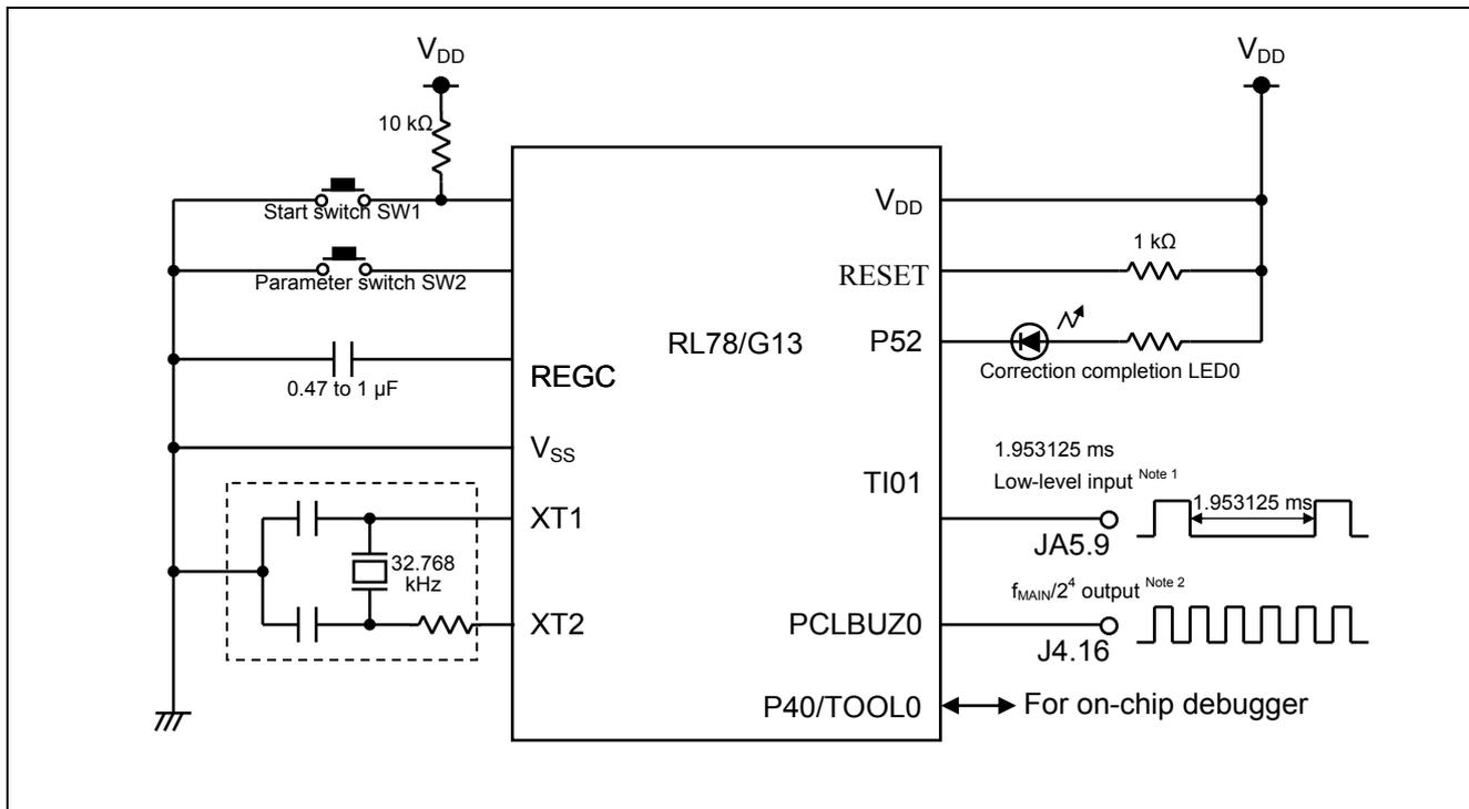
Figure 4.1 Hardware Configuration
