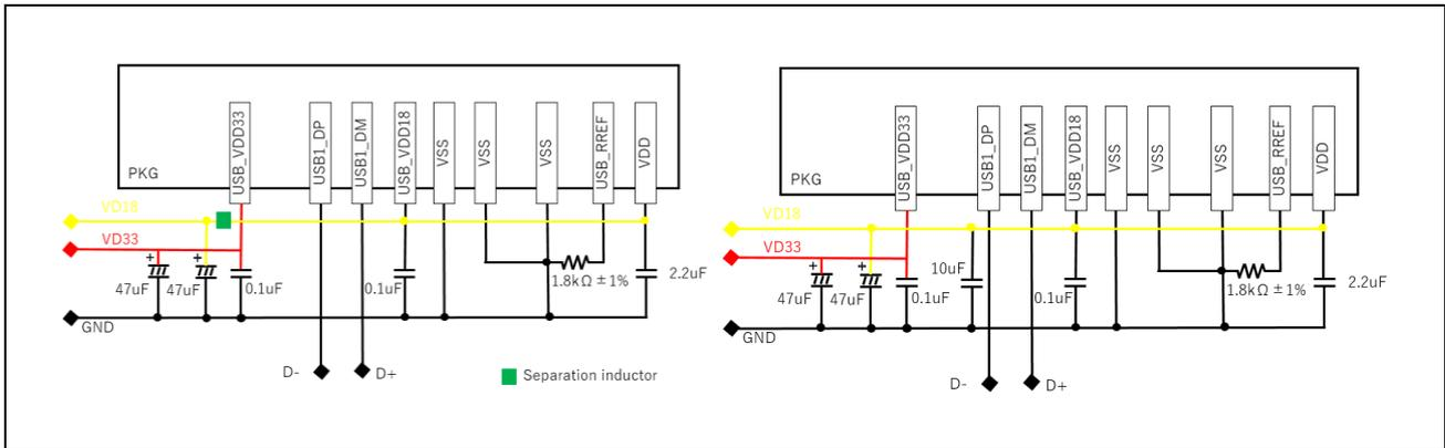
Figure B.1 Configuration of External Parts in the Case of 1 Port (left: with separation inductor, right: without separation inductor)
