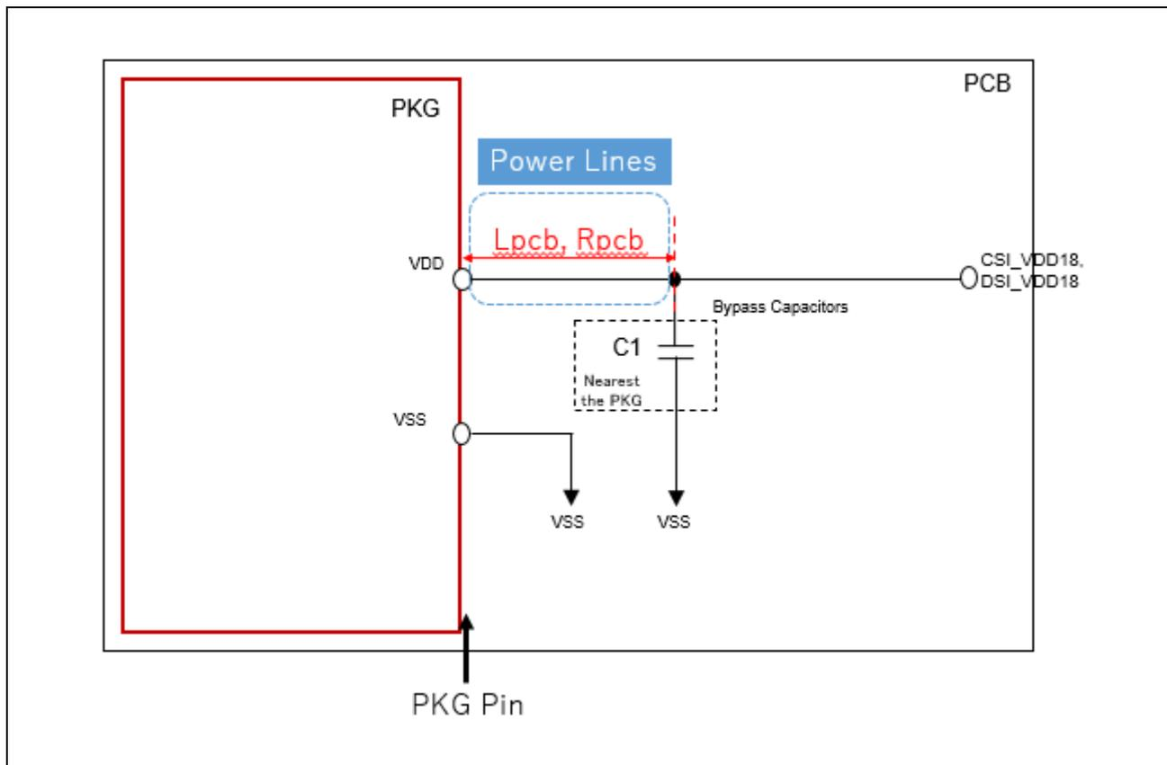
Figure 1.4 Power Line Topology of MIPI-CSI and MIPI-DSI
