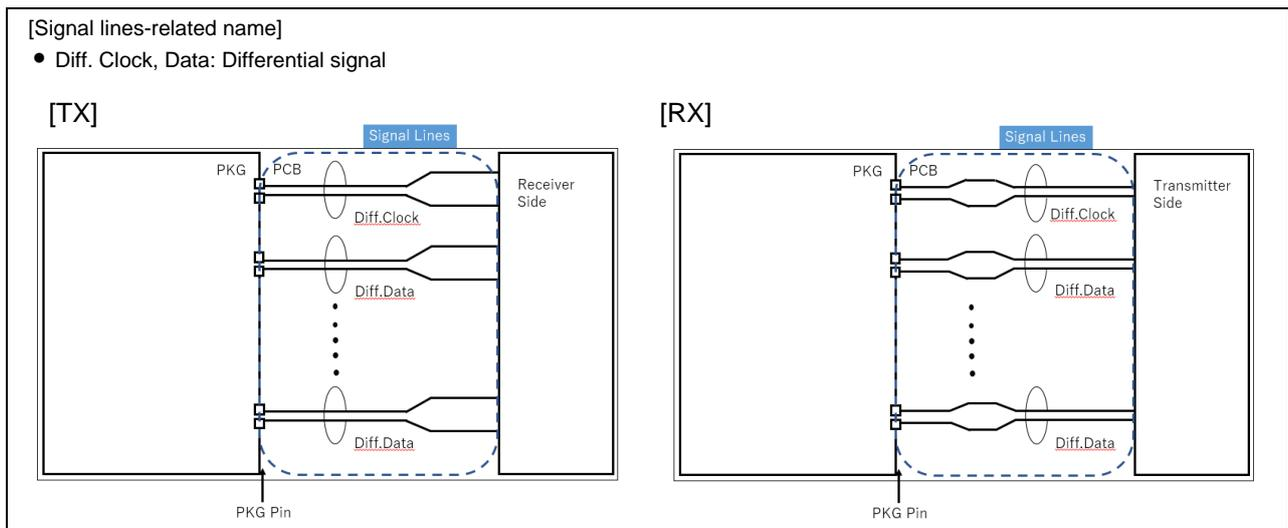
Figure 1.1 Signal Line Topology of MIPI-CSI and MIPI-DSI
