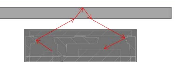
Figure 4. Example Optical Crosstalk Light Path from Top Surface of Cover Glass
